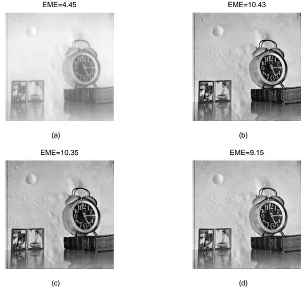
Fig. 3. Enhancement of the original image (a) via  $\alpha$ -rooting based on the Fourier (b), Hadamard (c), and cosine (d) transforms when  $\alpha = 0.92$ .
