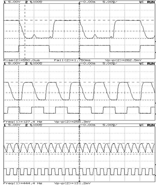
**Figure 11.** Raw output of photo detector for different CCR modulation frequencies. Direction of incident light is near  $(-1,-1,-1)$ . The square wave represents the input signal which modulates the CCR, where a low input pulls down the movable mirror. Actuation voltage is 15V.
