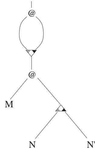
Here  $(M \_)$  is shared by the function and the argument of the top application; the hole is filled with  $N$  for the function and with  $N'$  for the argument.
