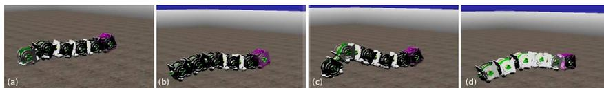
**Fig. 7** Evolved motion of several joined robot modules in the projects' 'Symbricator Simulator'. The hinges of joined modules are contracted in delayed oscillations by the evolved AHHS. A caterpillar-like motion pattern was finally evolved.
