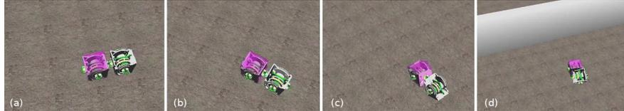
**Fig. 6** Evolved motion of two joined robot modules in the projects' 'Symbricator Simulator'. The hinges of the two modules are contracted in an oscillations by the evolved AHHS. This pushes the organism forward.
