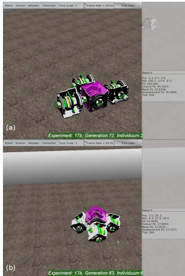
**Fig. 8** Two different motion patterns evolved successively with the same body shape. a: flat body, oscillators move peripheral hinges like fins. b: erected posture of the organisms, peripheral robots moved like legs.
