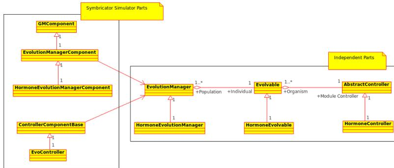
**Fig. 3** Software design of our AE framework. It is embedded into the projects’ ‘Symbicator Simulator’ which is based on the Delta3D open-source gaming/simulation engine [22].
