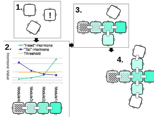
**Fig. 5** The development of the body formation in an EMMR. The process of the progress from single module formation in a swarm to robot organism with legs is depicted in four steps. One possible way of achieving this with our AHHS is denoted as a schematic graph of hormone values of two hormones in step 2. For further explanation see text.
