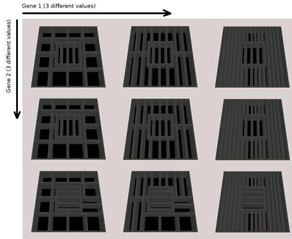
**Fig. 4** Internal compartmentalization of the robot. This important structural feature in an AHHS controller is mutated by altering ‘layout rules’. This figure shows 9 configurations that result from a combination of mutations of 2 genes (rules).
