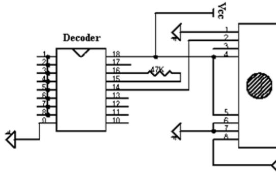
**Figure 6:** Hardware connection of Manchester Encoder with transmitter.
