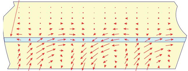
Figure 3 — Actual magnetization pattern recorded on tape (after Tjaden and Leyten)<sup>5</sup>
