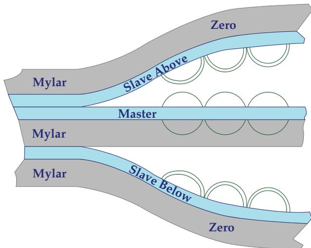
Figure 4 — Contact printing (and, with upper tape inverted, print-through) configuration.
