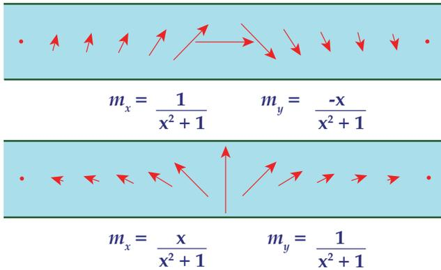
Figure 2 — Two magnetization patterns yielding one-sided fluxes. No flux exists above the planes.
