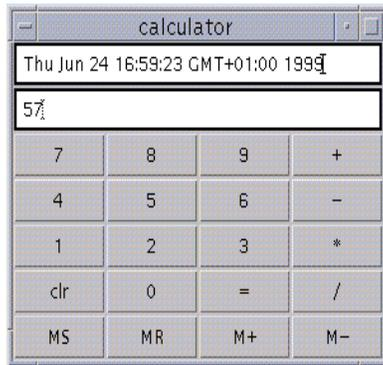
The GUI is implemented as a Java agent; the calculations and memory are implemented as an EBG agent. Events are generated by AWT buttons causing messages to be sent from the Java agent to the EBG agent. Part of the EBG agent is shown in figure 4. The `op1` behaviour handles operations for the left hand operator and `op2` for the right. `n` is the current number and `m` is the memory.
