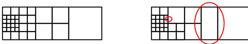
Figure 4. A one-irregular grid with ‘hanging’ nodes (left) and a grid which contains several mistakes (right) indicated by the circles.
