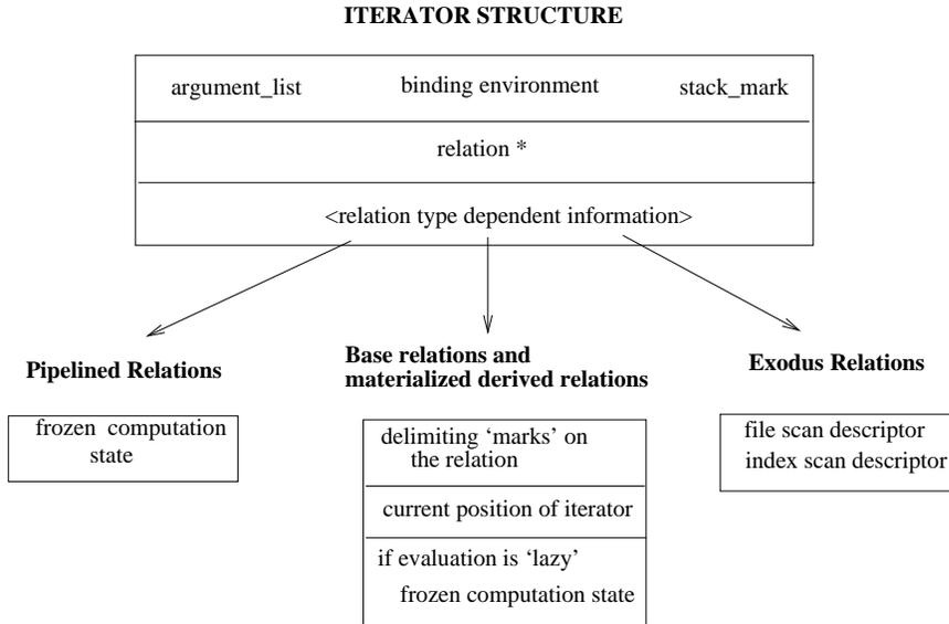
Figure 6: The TupleIterator Structure
