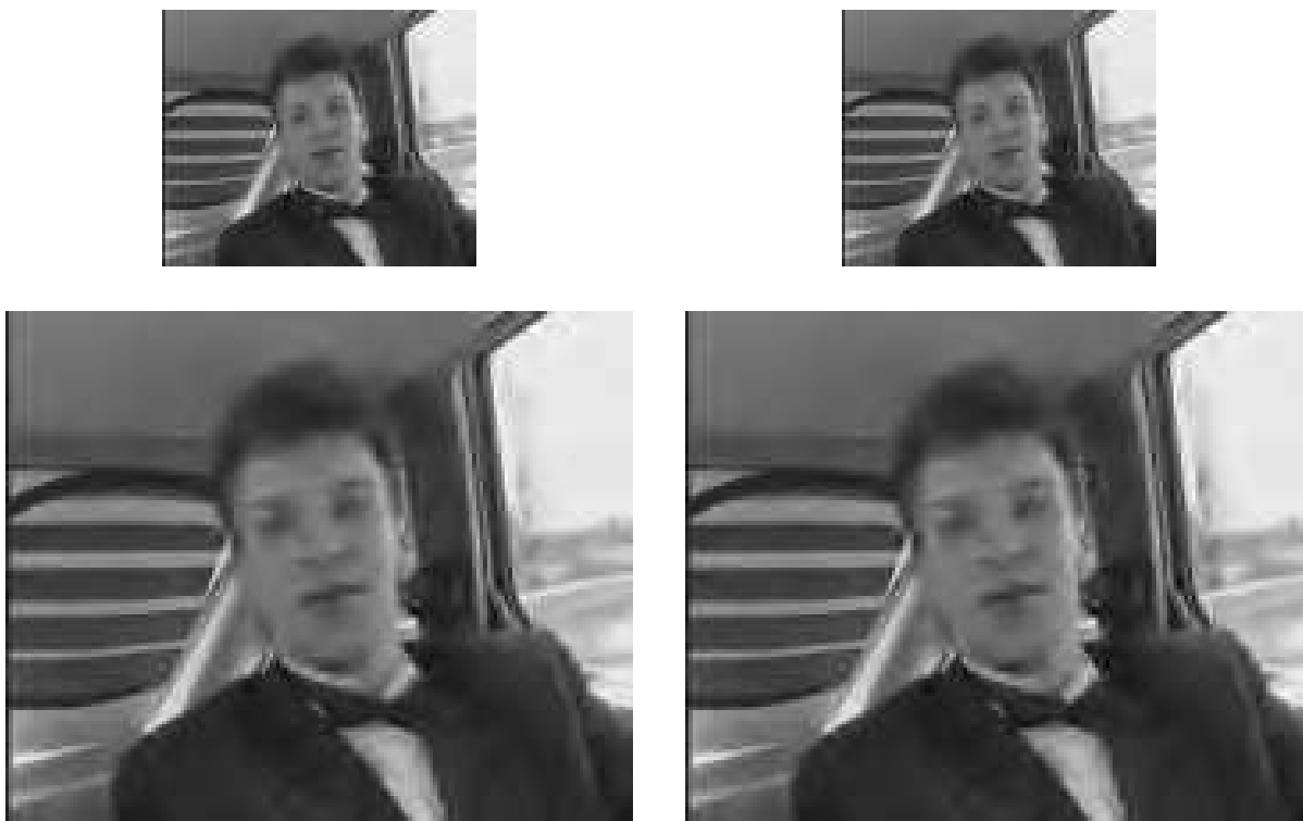
Figure 16: Multiresolutional decoded frame 0 of “Carphone” sequence with the embedded 3D SPIHT video coder (a)Top-left: spatial half resolution ( 88 \times 72 and 10 f/s) (b)Top-right: spatial and temporal half resolution ( 88 \times 72 and 5 f/s) (c)Bottom-left: temporal half resolution ( 176 \times 144 and 5 f/s) (d)Bottom-right: full resolution ( 176 \times 144 and 10 f/s).
