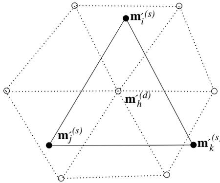
Fig. 2. Illustration of the relations of the model vectors in a sparse ( $s$ , solid lines) and dense ( $d$ , dashed lines) grid. Only partial grids are shown in the figure. Here  $\mathbf{m}_h^{(d)}$  shall be interpolated in terms of the three closest “sparse” models  $\mathbf{m}_i^{(s)}$ ,  $\mathbf{m}_j^{(s)}$ , and  $\mathbf{m}_k^{(s)}$ , respectively.
