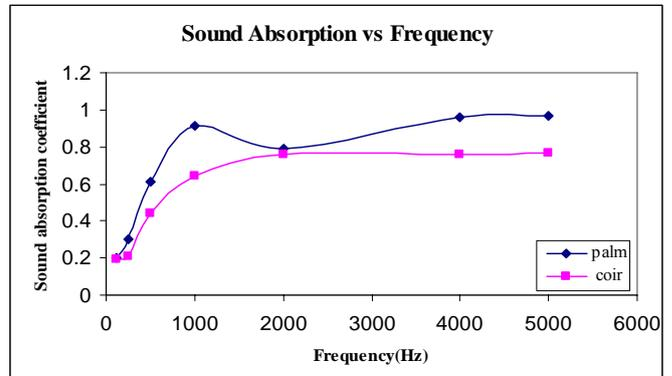
Fig. 3: Sound Absorption Coefficient versus Frequencies of Coir fiber and Oil Palm fiber [7]
