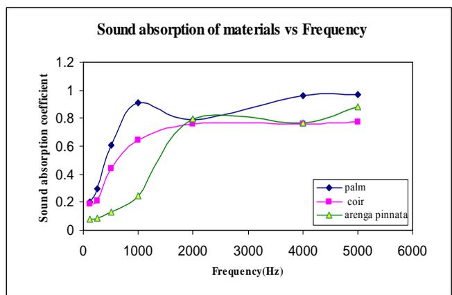
Fig. 4: Sound Absorption Coefficient versus Frequencies of palm, coir, and *Arenga pinnata* fiber
