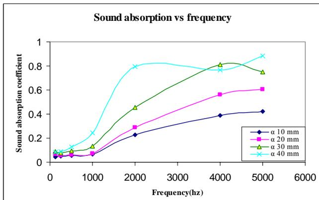
Fig. 2: Sound absorption of *Arenga pinnata* fiber
