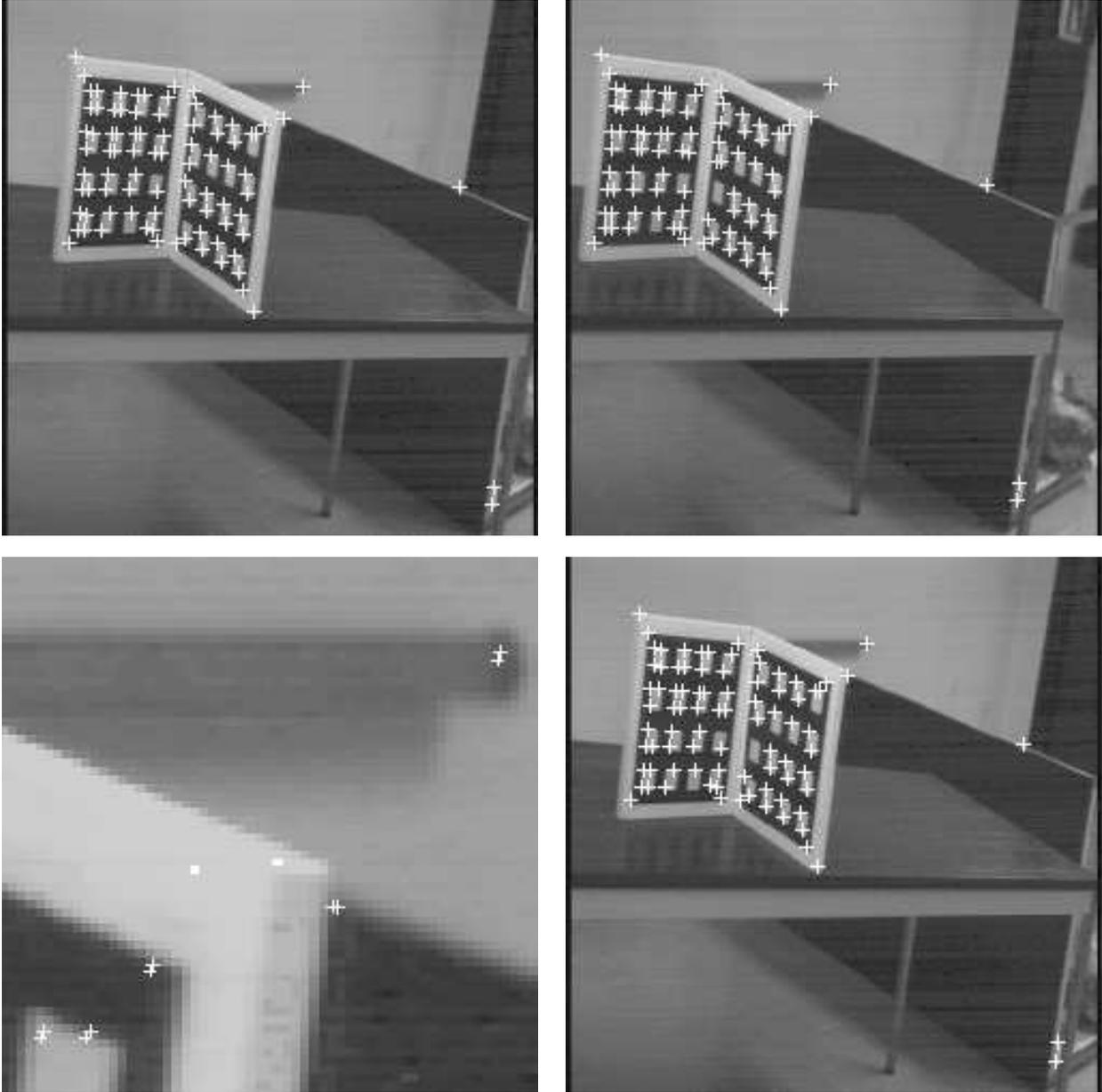
Figure 14: Actual matches (top), and matches predicted by the homography (bottom).
