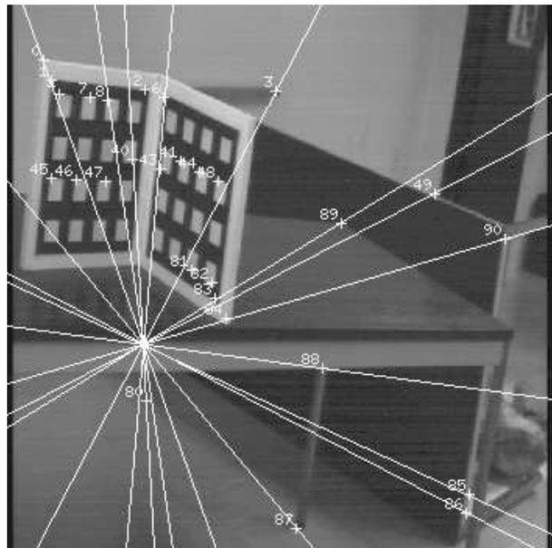
Figure 15: Ambiguity: four coherent epipolar pencils in the first image.
