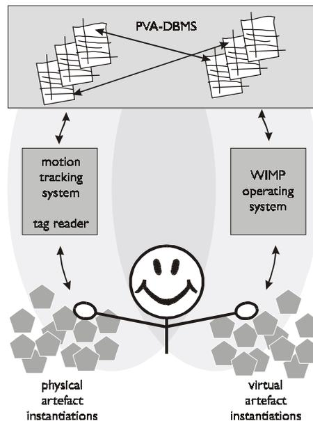
**Figure 2:** Magic Touch architecture outline. The PVA-DBMS linking the physical (left) and virtual (right) environments together by keeping track of artefact instantiation changes done by the user in any of the two environments.
