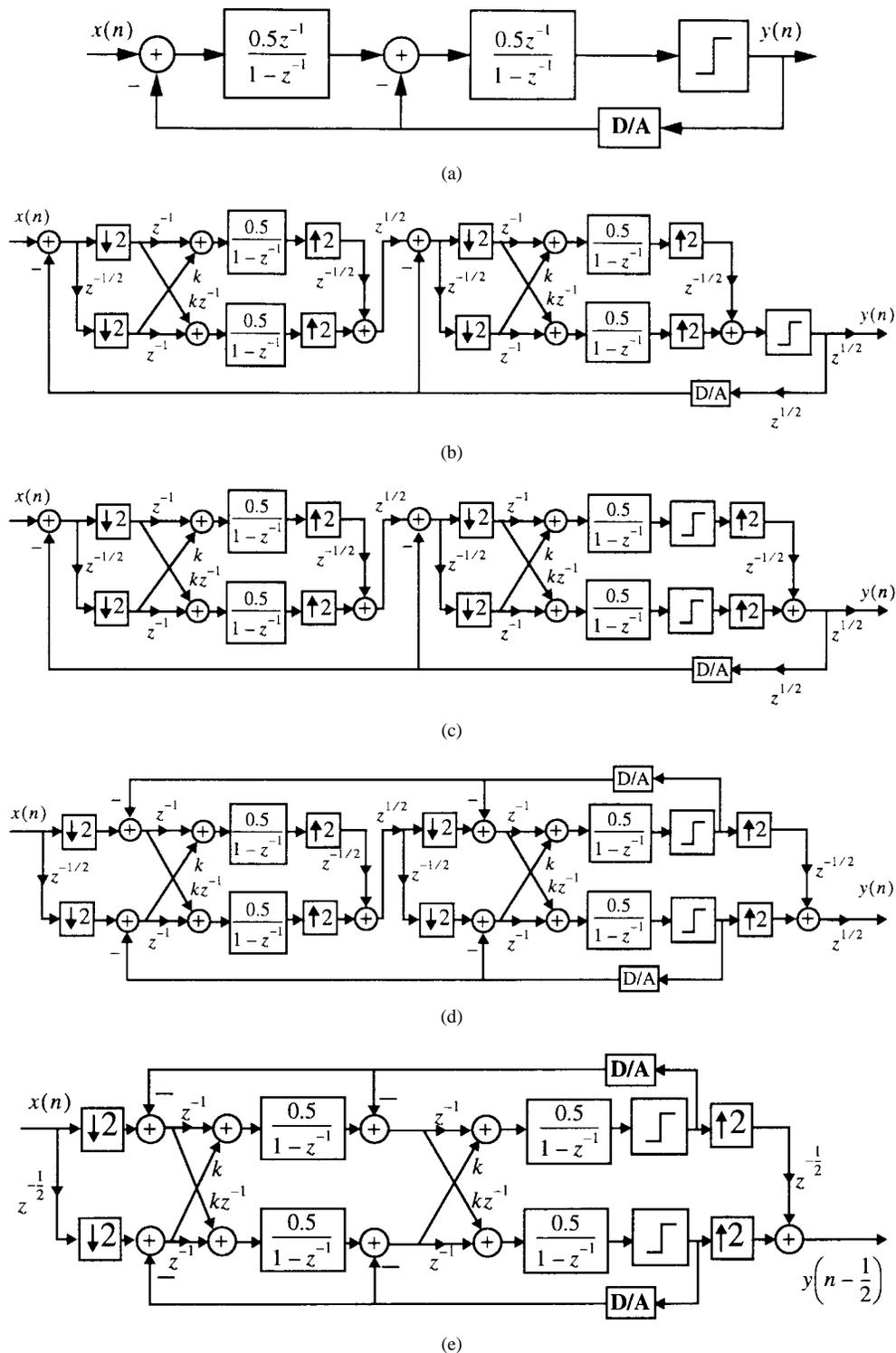
Fig. 6. Second-order  $\Delta\Sigma$  modulator. (a) Conventional. (b) With block digital equivalent filters. (c) With quantizers in the lower-rate section. (d) With D/A's in the lower-rate section. (e) Final TIM structure. Note that  $k = 1$ .
