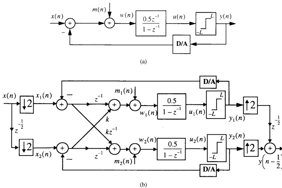
Fig. 10. First-order  $\Delta\Sigma$  modulator. (a) Conventional. (b) TIM.
