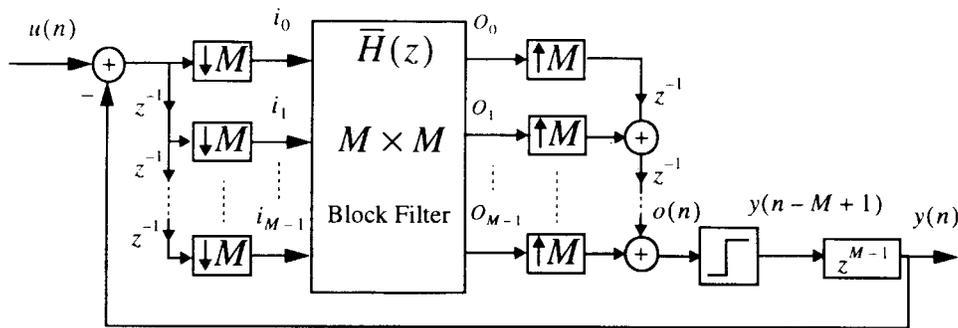
Fig. 3. Oversampling converter with a block digital filter.
