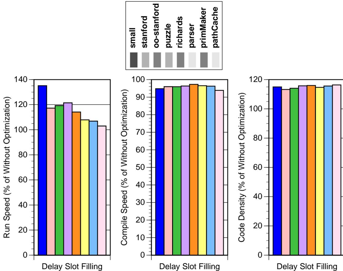
Filling delay slots on the SPARC speeds up the benchmarks by between 5% and 35%, costs little in compile time, and reduces compiled code space requirements by almost 15%.\* Given these execution speed and compiled code space benefits, delay slot filling seems to be worth its nominal compile time expense.
