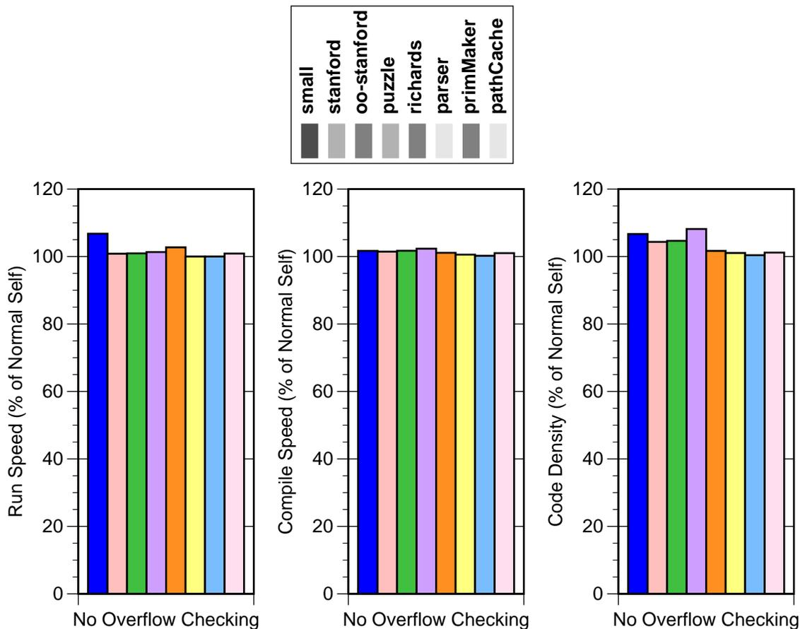
Overflow checking slows execution by less than 5% for all but the smallest benchmarks. However, since the register allocator frequently leaves an extra register move behind even when overflow checks are removed, the cost of overflow checking may be understated by these results by up to a factor of two. Overflow checking imposes negligible compile-time cost and a small space cost.
