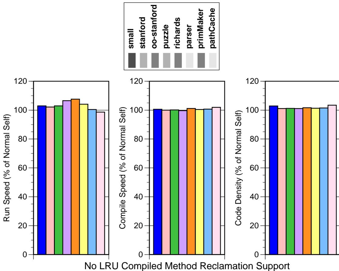
LRU support imposes a run-time cost of up to 8% over a system without this support. This cost is directly proportional to the call frequency of the program being measured. LRU reclamation support takes little additional compile time and little additional compiled code space.
