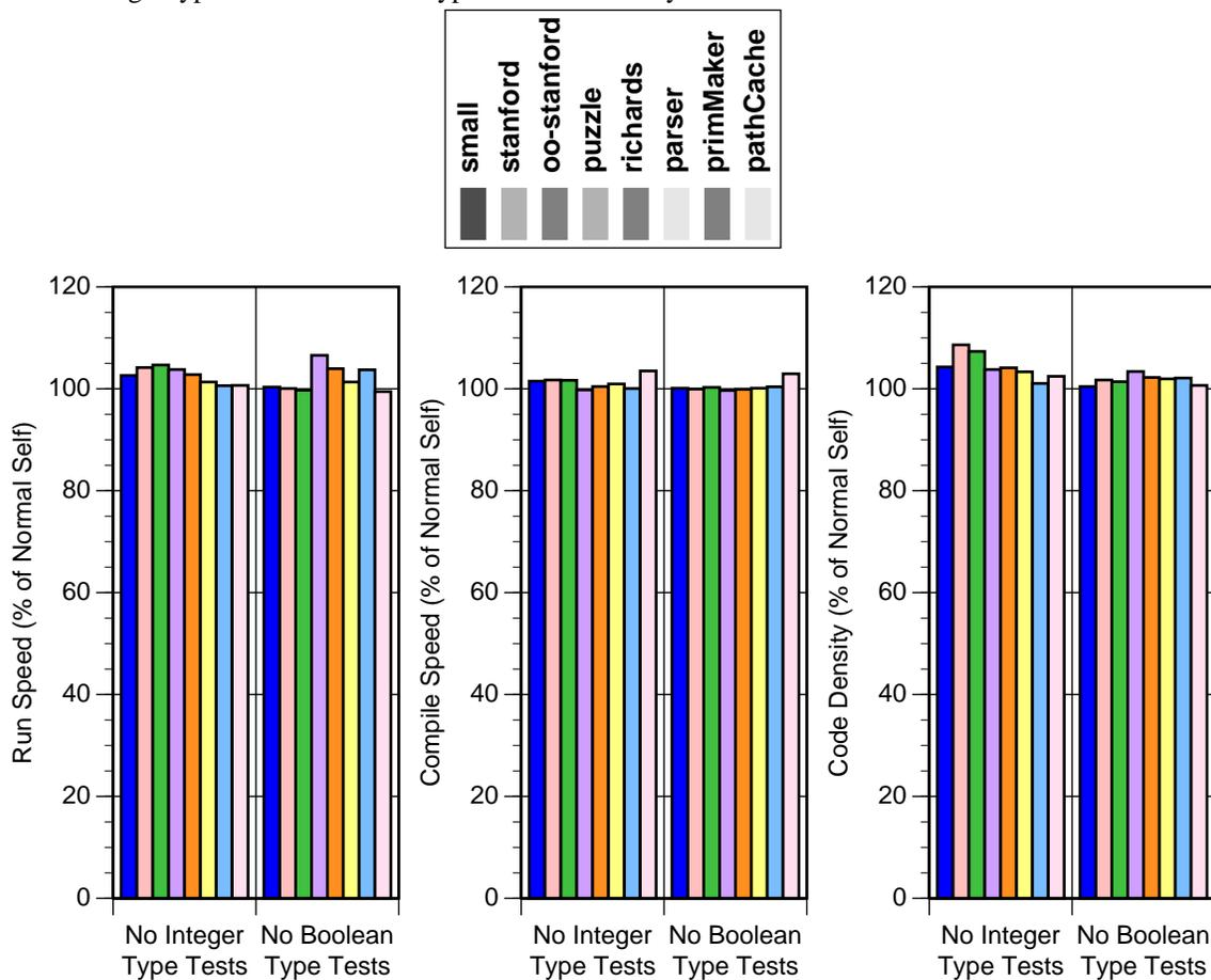
Type tests increase execution time by no more than 10% for these benchmarks, take up little extra compile time, and add no more than 10% additional compiled code space. Type analysis, splitting, and lazy compilation of uncommon cases are largely responsible for the relatively low number of type tests that remain in compiled SELF code.
