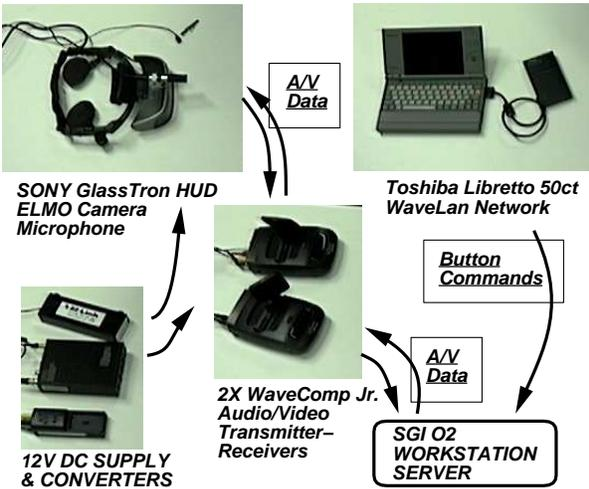
Figure 5: The Wearable Hardware System
