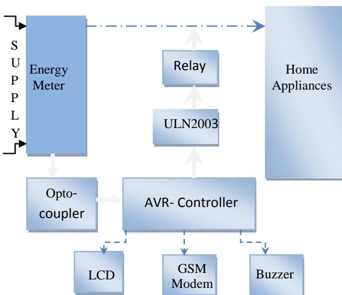
Fig 2. Circuit descriptions of AVR Microcontroller
