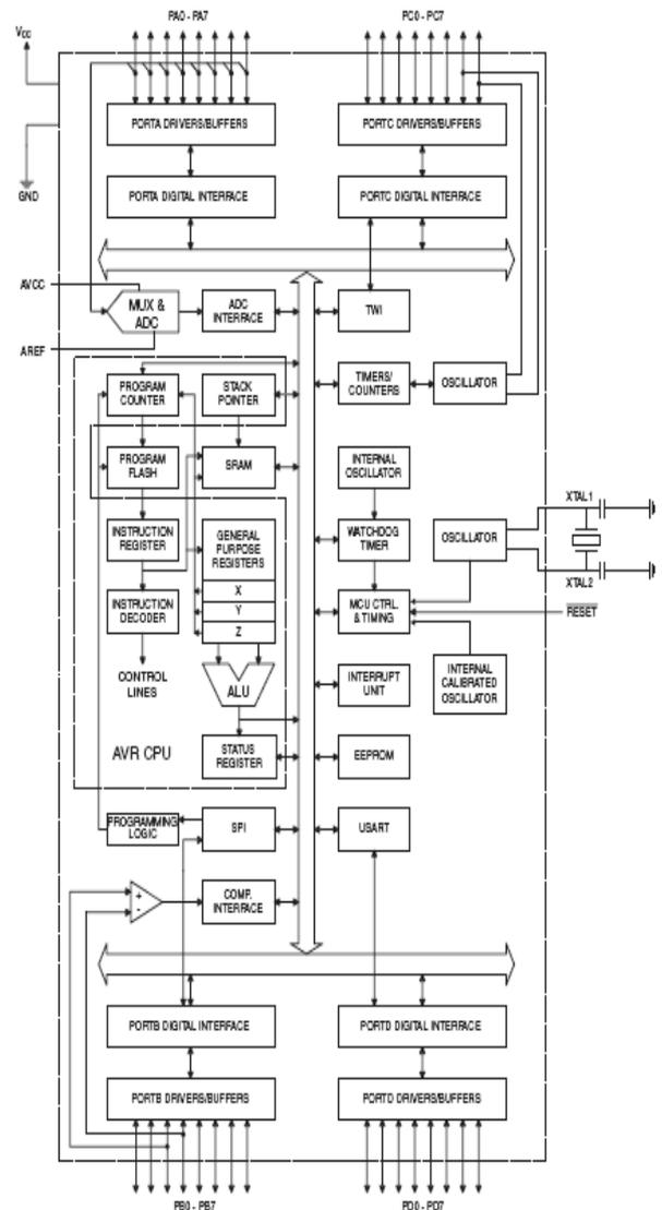
Fig 1. Internal Architecture of AVR Microcontroller
