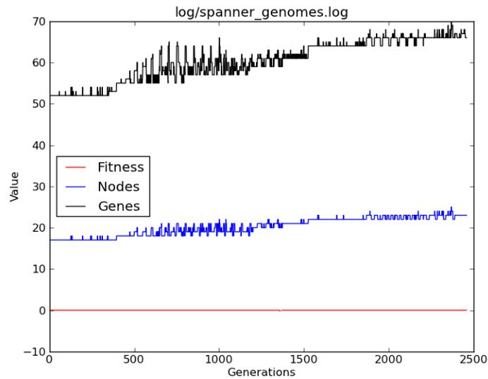
Figure 5: This plot shows an evolution run, attempting (and failing) to train the neural network controller to imitate the simple PID controller.
