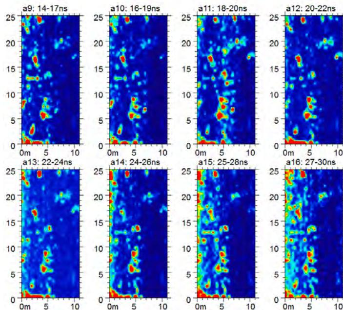
Fig.5: Time-Slice of Area 1 at 0ns- 37ns with 500 MHz antenna
