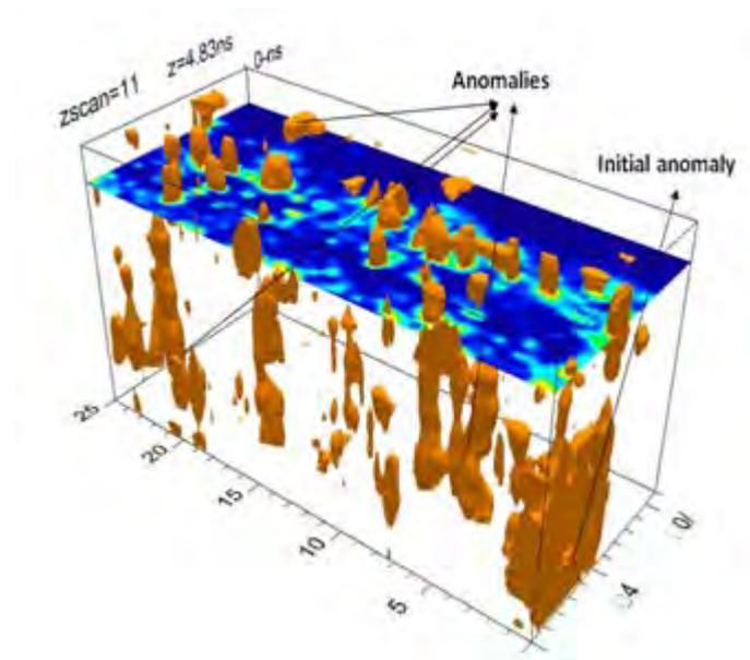
Fig.7: GPR-slice iso-surface renders and times-slices obtained in the time windows 3-37ns with 500 MHz antenna
