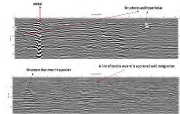
Fig.8: Processed radargrams (Area 3) (B-scan) achievement with 500 MHz from line 10 (a) and with 800 MHz antenna from line 10 (b).
