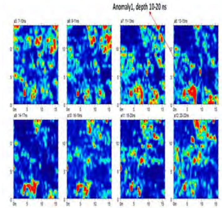
Fig.9: Time-Slice of Area 1 at 7ns- 22ns with 500 MHz antenna
