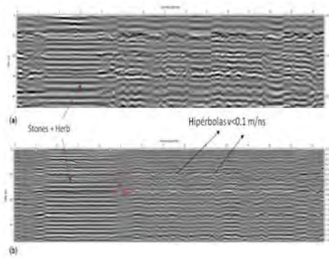
Fig.2: Processed radargrams (Area 1) (B-scan) achievement with 500 MHz from line 32 (a) and with 800 MHz antenna from line 33 (b).
