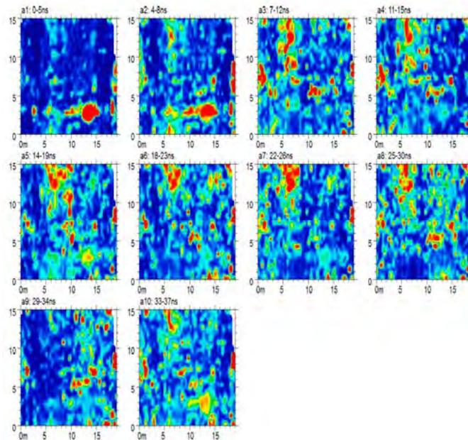
Fig.3: Time-Slice of Area 1 at 0ns- 37ns with 500 MHz antenna
