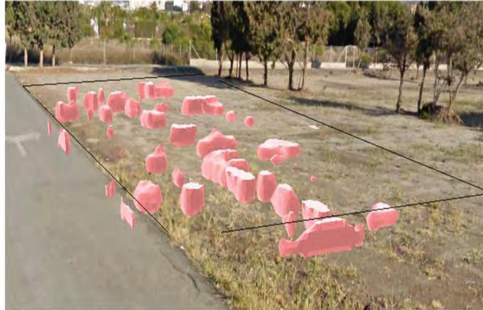
Fig.6: Isosurface of anomalies at  $T < 15\text{ns}$  with 500 MHz antenna
