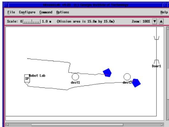
Fig. 33. *MissionLab* showing the operator console after execution of a simple two robot mission. The robots start on the left edge of the lab and proceed to the *dest1* point in line formation. They then continue to location *dest2* using column formation. They are shown in their final positions, with the trails marking the path they each traversed.
