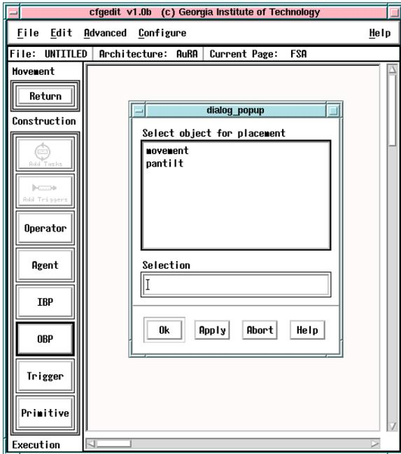
Fig. 14. *CfgEdit* menu to pick output binding point
