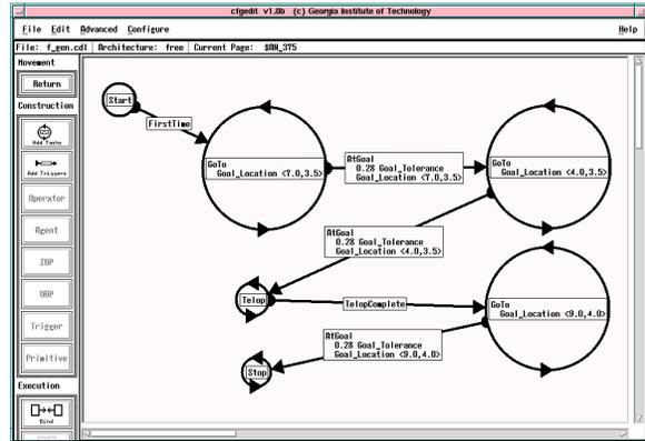
Fig. 23. Generic configuration suitable for binding to either architecture
