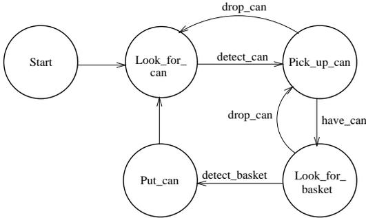
Fig. 7. FSA for a trash collecting robot
