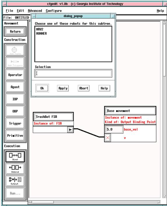
Fig. 20. The robot selection menu, presented during binding
