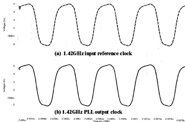
Fig. 15 1.426 GHz input reference and PLL output clocks.
