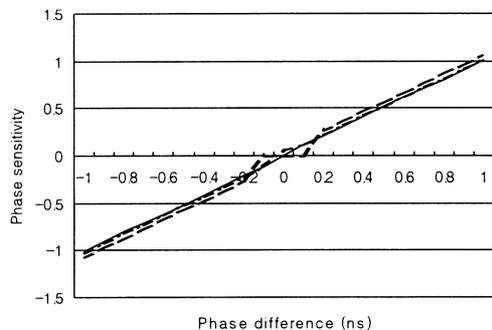
**Fig. 8** Phase characteristics of the pt-type PFD (long dashed-line), and nc-type PFD (short dashed-line), and our PFD (type-2) (solid line).
