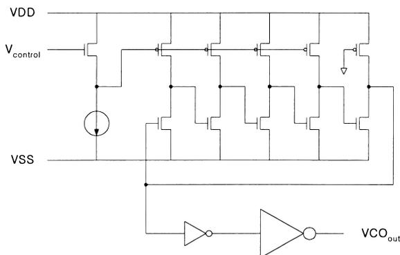
Fig. 13 Circuit schematic of VCO [6].
