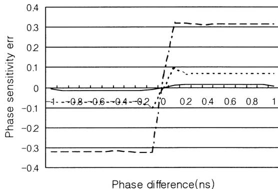
**Fig. 9** Phase sensitivity error of the pt-type PFD (short dashed-line), and nc-type PFD (long dashed-line), and proposed PFD (solid line).
