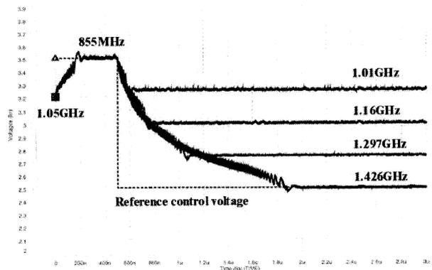
Fig. 14 Response of a third-order PLL for various input reference step variation.
