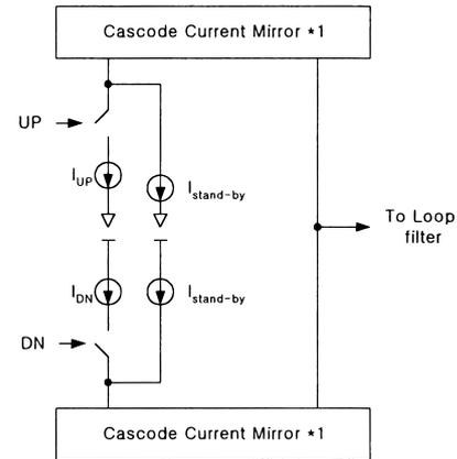
Fig. 6 Block diagram of our charge-pump.
