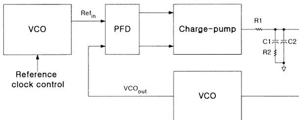
Fig. 12 Block diagram of a third-order PLL.
