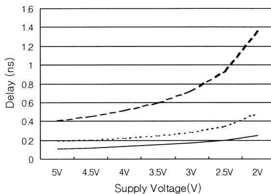
**Fig. 10** Setup delay (solid line PFD type 1 and type 2) and reset delay of proposed PFD (PFD type 1 : short dashed line, PFD type 2 : long dashed line) as a function of supply voltage.
