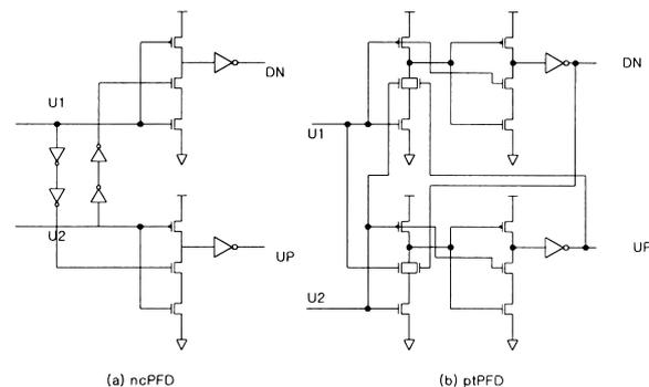
Fig. 2 Circuit schematic of dynamic PFDs [2],[3].
