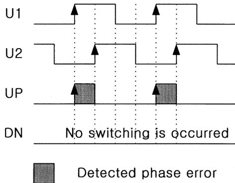
Fig. 5 The operation of the proposed PFD.
