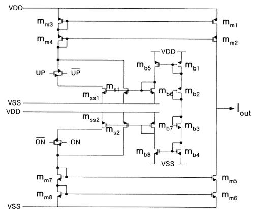
Fig. 7 Detailed circuit schematic of our charge-pump.
