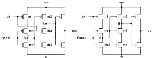
(a) Proposed D flip-flop 1 (b) Proposed D flip-flop 2
