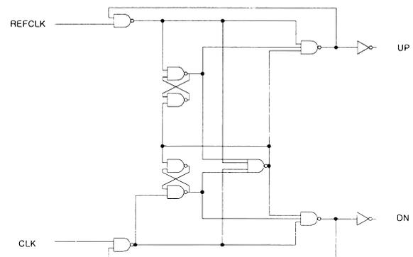
Fig. 1 A conventional CMOS PFD [1].
