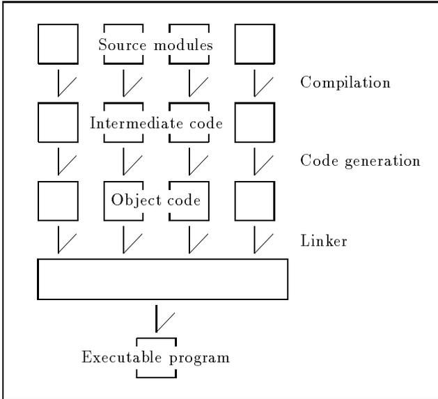
Figure 5: Standard approach to separate compilation
