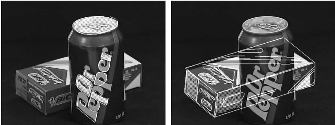
Figure 15: These figures show the performance of the system on more realistic objects. On the left, the system uses the forward constraints to accurately determine the pose of the soda can. Four regions are used in this case. The regions are surface markings on the cylinder of the can, and a circular region from the top of the can. On the right, the backward constraints are used to locate the pen box. Note that the soda can is occluding some of the regions used.
