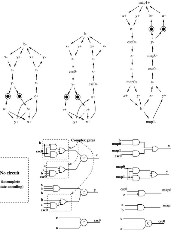
Figure 4: State encoding and technology mapping
