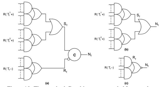
Figure 10: The standard-C architecture extended for complex gates
