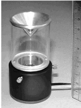
Figure 10: 360°-camera with conical mirror (scale in cm)
