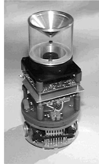
Figure 11: Khepera<sup>TM</sup> robot with camera and conical mirror.
