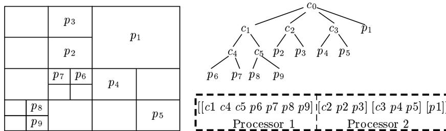
Fig. 1. Example of a Barnes-Hut tree and its representation as a vector.
