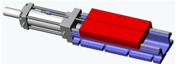
Fig. 4 Pneumatic sliding unit with course adjustment.
