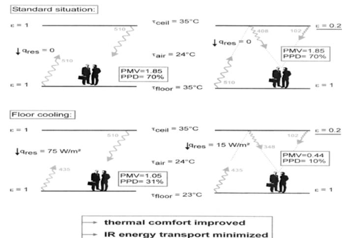
**Figure 1** The effect of low emission IR coating.
