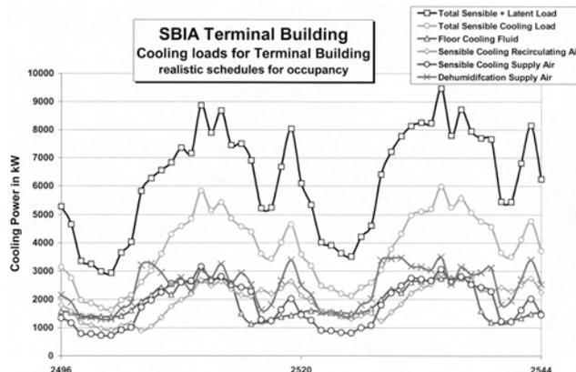
Figure 5 SBIA terminal building cooling loads.
