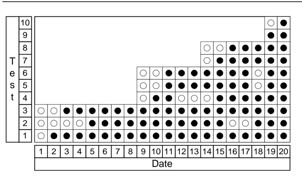
When we look at this chart, we see blocks of tests coming on line. It takes a day or so before they run right, but then usually they continue to run right along. But something happened to test 4 on the 12th, and to test 2 on the 16th, and to 5 and 6 on the 18th. These changes, especially blocks of changes
