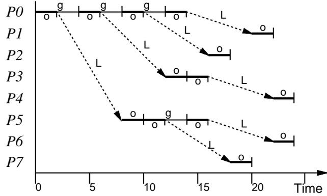
Figure 3: *Optimal broadcast tree for  $P = 8, L = 6, g = 4, o = 2$  (left) and the activity of each processor over time (right). The number shown for each node is the time at which it has received the datum and can begin sending it on. The last value is received at time 24.*
