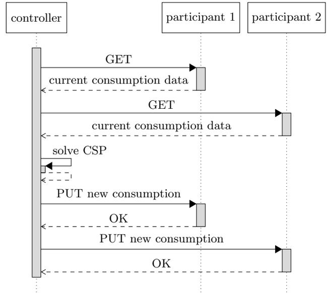
**Figure 3: Communication flow of one controller with two participants.**
