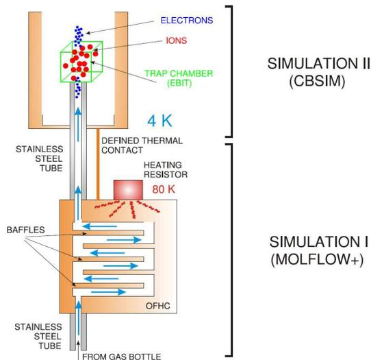
Figure 1: Schematic view of the cold gas source (bottom) and the attached ionization chamber (top) where the gas atoms are ionized by electron impact ionization. The structure shown is a few cm high.
