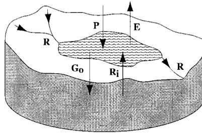
Figure 3. Schematic diagram of the hydrological balance of a lake system. Where R = Runoff, D = Discharge, P = Precipitation, E = Evaporation,  $G_i$  = groundwater Inflow, and  $G_o$  = Groundwater Outflow. For a closed system in equilibrium conditions,  $D = G_i = G_o = 0$  (modified after Mason *et al.*, 1994)
