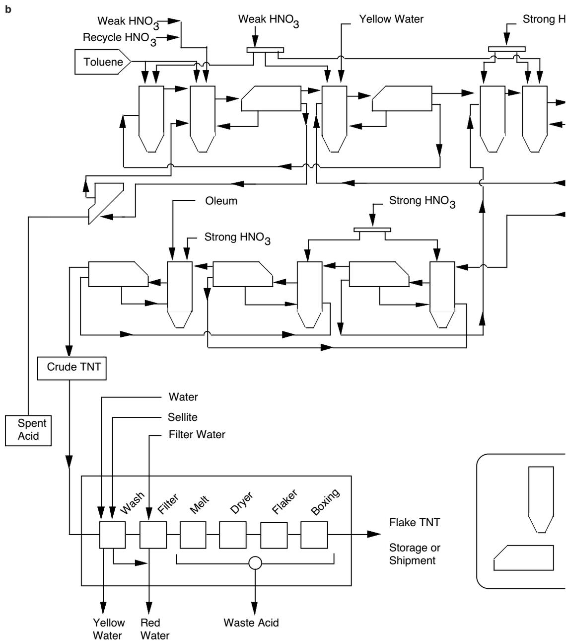
in anhydrous sulfuric acid) to form crude TNT. The crude TNT then undergoes a series of washes to remove crude unreacted toluene, MNT, and DNT. Reprinted from US Army Environmental Hygiene Agency. *Water Pollution Aspects of Explosive Manufacturing*. Aberdeen Proving Ground, Md: USAEHA; 1985. USAEHA Technical Guide 140; (a) p 16, (b) pp 28, 30.
