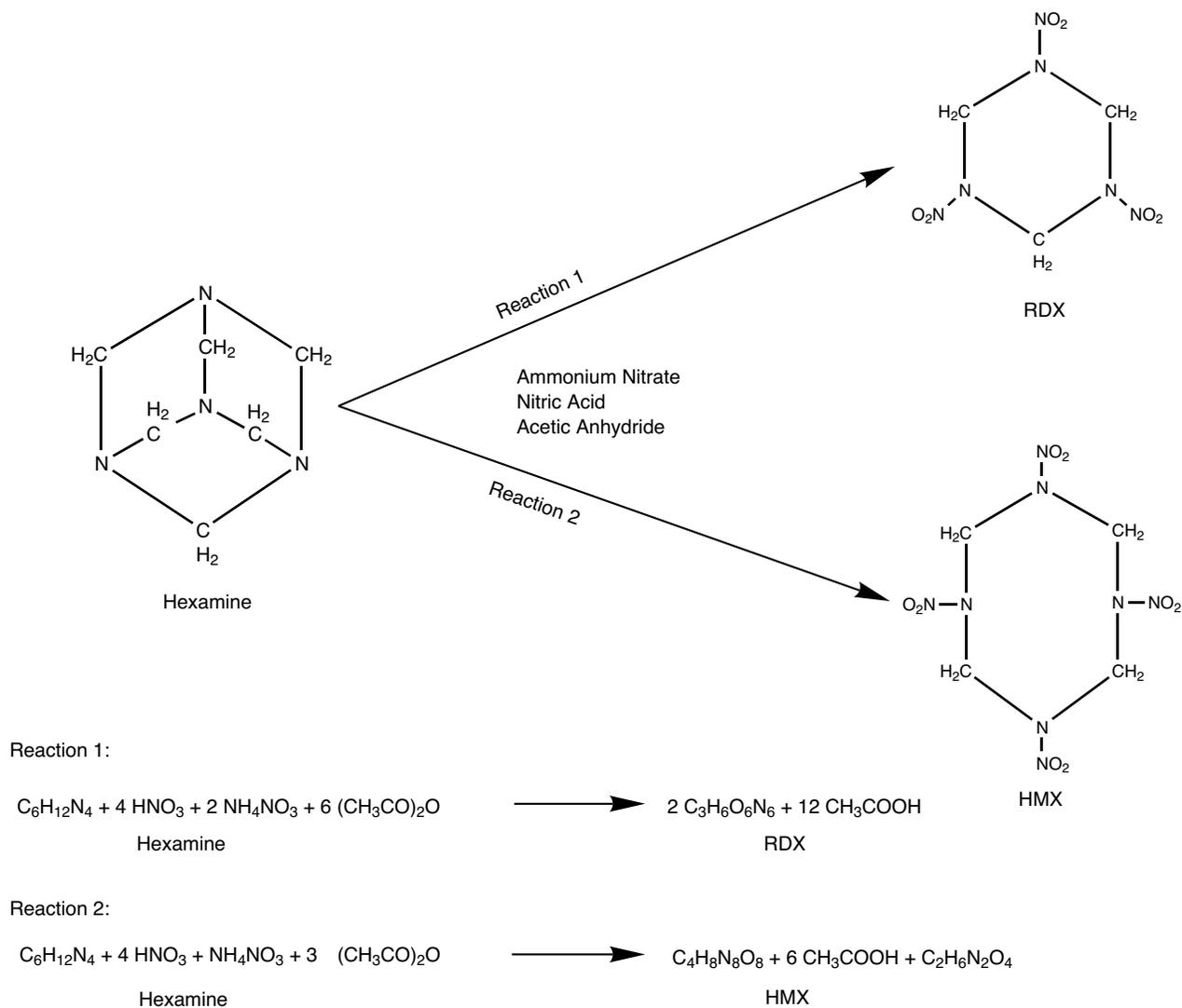
**Fig. 9-16.** The chemistry of RDX and HMX production. HMX is an unavoidable coproduct of the production of RDX from hexamine. Most RDX preparations contain at least 9% HMX. Reprinted from US Army Environmental Hygiene Agency. *Water Pollution Aspects of Explosive Manufacturing*. Aberdeen Proving Ground, Md: USAEHA; 1985: 21. USAEHA Technical Guide 140.
