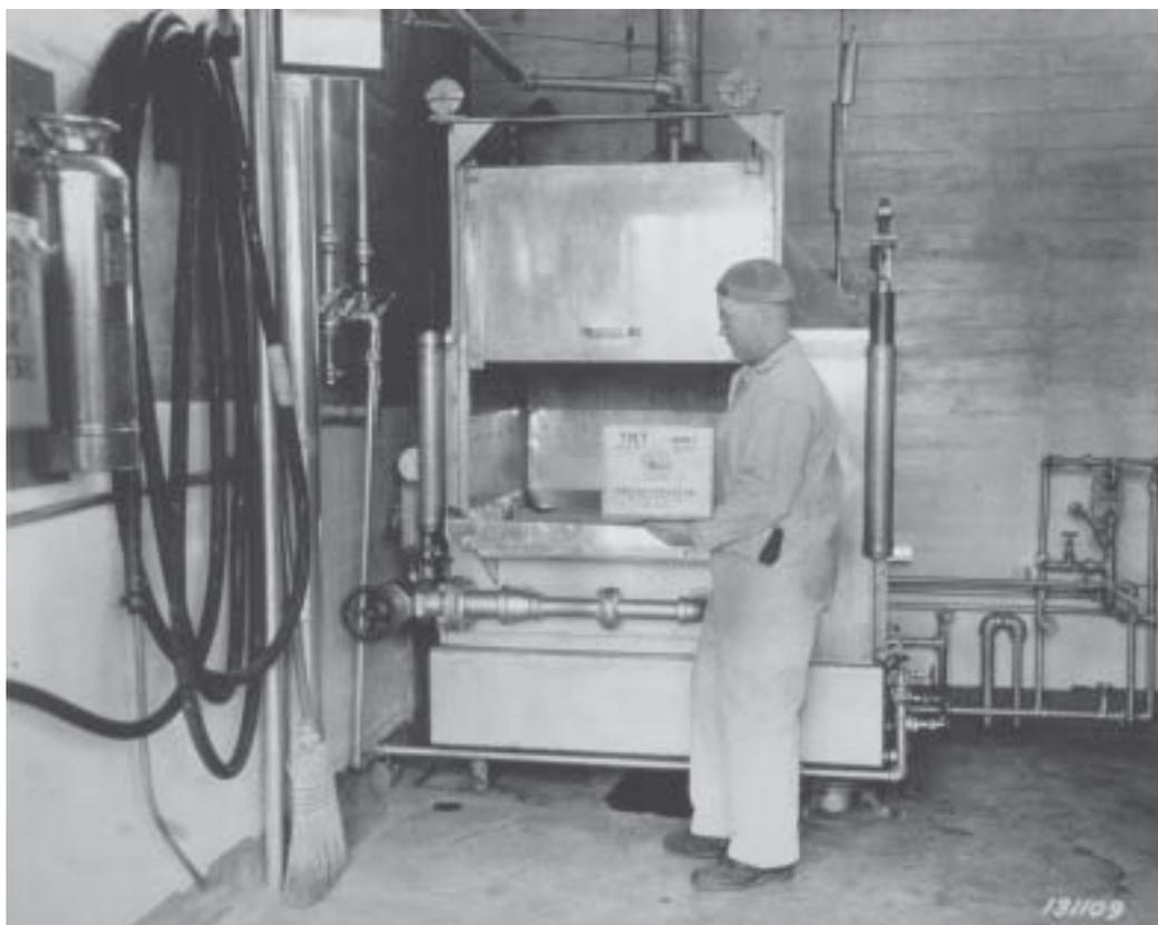
**Fig. 9-7.** This photograph is dated April 1942. A worker is preparing to dump a box of bulk TNT into the melt unit, through which steam is passed. The liquified TNT will then be poured into shells and bombs. The worker wears special nonsparking safety shoes made without nails. Photograph: Courtesy of the Ordnance Department, Signal Corps College; Ordnance Center, Picatinny Arsenal, New Jersey.
