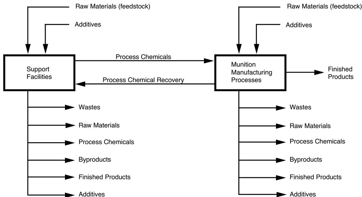
Fig. 9-5. Simplified flow for munition manufacturing processes. Adapted from US Army Environmental Hygiene Agency. *Water Pollution Aspects of Explosive Manufacturing*. Aberdeen Proving Ground, Md: USAEHA; 1985: 5. USAEHA Technical Guide 140.
