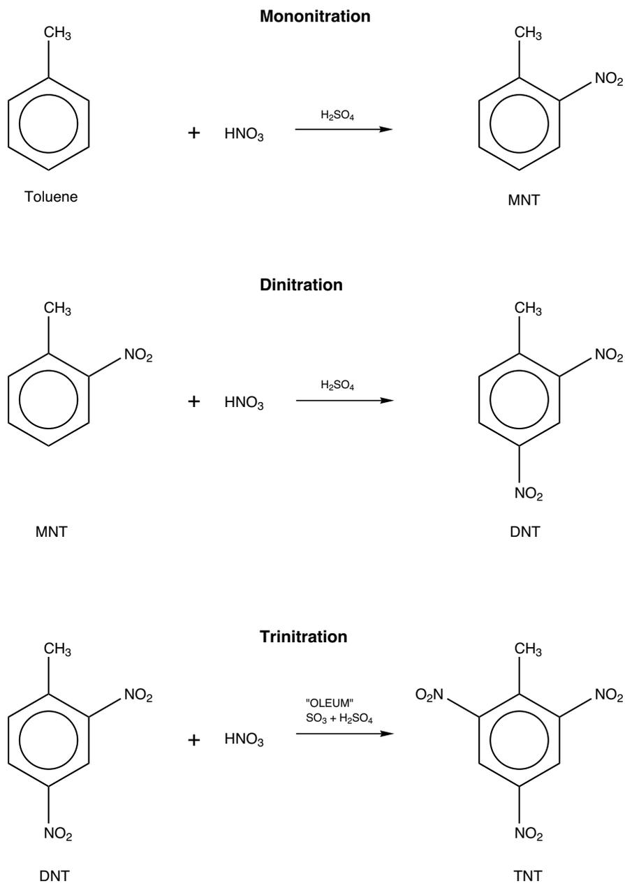
**Fig. 9-14.** The trinitration of toluene: (a) chemical synthesis and (b) industrial (enclosed) process stream. In the manufacture of TNT, toluene is first reacted with nitric acid to form mononitrotoluene (MNT), which is then pumped to another area, where it is reacted with nitric acid (under different reaction conditions) to form dinitrotoluene (DNT). The DNT is then pumped to yet another area where it is reacted with oleum (a solution of sulfur trioxide dissolved
