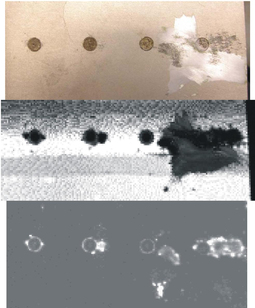
**Figure 21-5: From Top to Bottom: A Photograph, a UT Image, and an IR Image of a Section of Wing Plank from a Boeing 707, Showing Exfoliation Damage and Grinding Marks from Repairs – the material is 7178-T6 aluminum (from Forsyth et al. [24]).**
