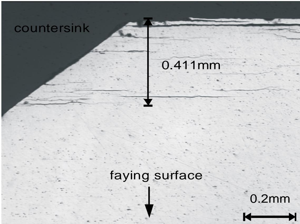
**Figure 21-4: Metallographic Section Around a Fastener Hole in a Boeing 707 Wing Skin Plank, Showing Multiple Layers of Intergranular Attack from Pits in the Countersink – the material is 7178-T6 aluminum (from Forsyth et al. [24]).**
