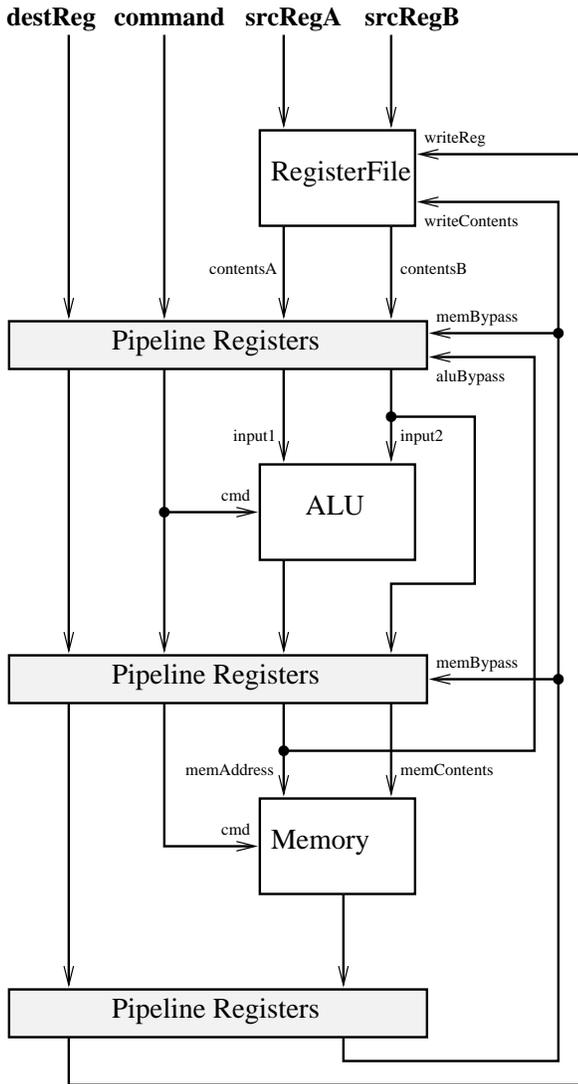
Figure 5: Block diagram of extended SHAM pipeline. Each *Pipeline Register* circuit is made up of multiple *Delay* and *Select* circuits. The *Select* circuits are used for bypassing, ensuring that the source operands are up-to-date.
