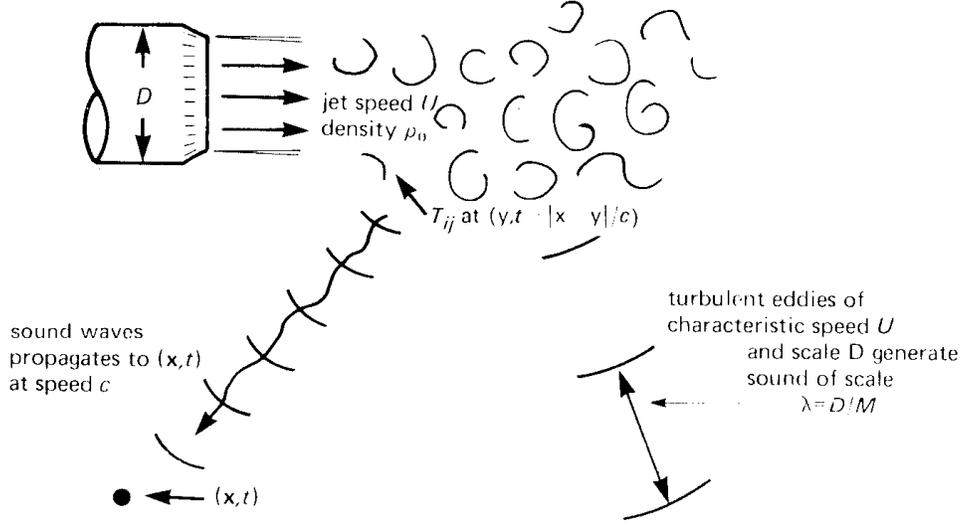
Figure 5: Sound generation by a low Mach number jet.
