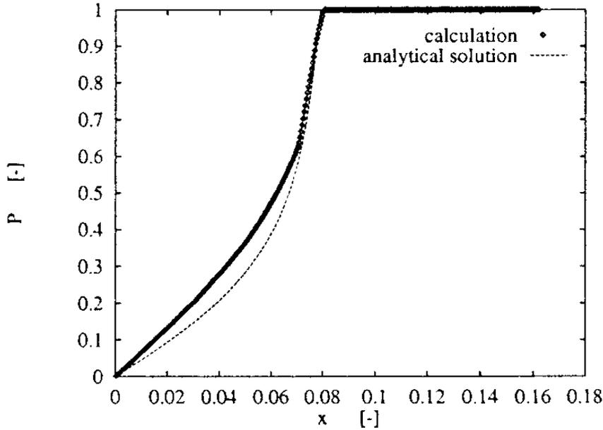
Figure 15: Pressure at a time instant for  $M = 10^{-2}$ ,  $\diamond$ : computed result with conservative formulation and single precision, dashed line: analytical solution.
