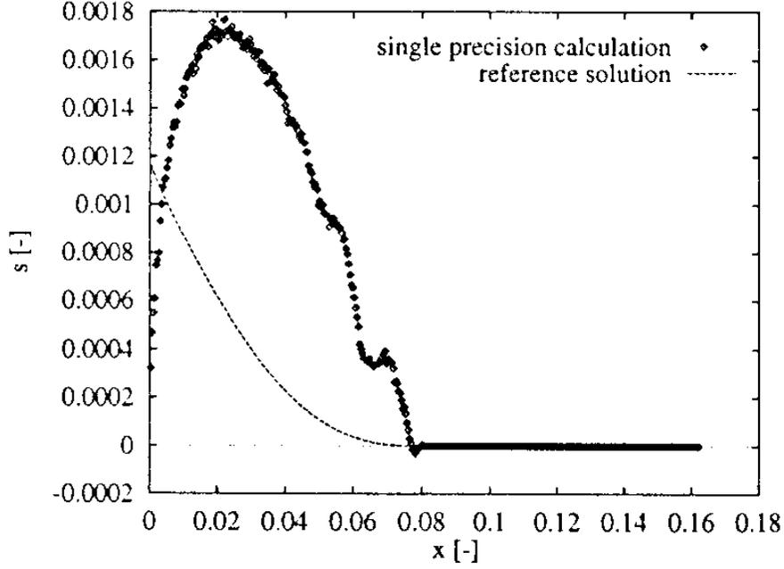
Figure 16: Entropy along the axis of the tube at a time instant for  $M = 10^{-2}$ ,  $\diamond$ : computed result with conservative formulation and single precision, dashed line: reference solution with double precision.
