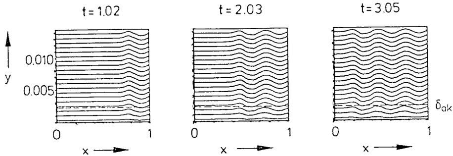
Figure 6: Acoustic velocity  $u'$  at different  $y$  locations in laminar flat plate boundary layer.
