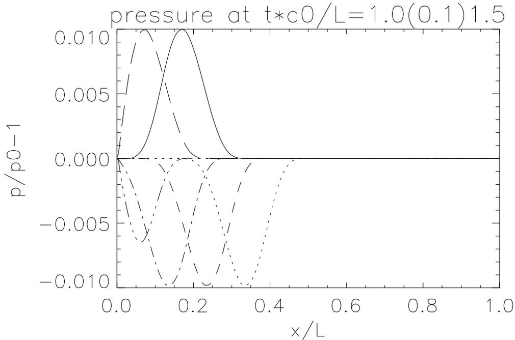
Figure 8: Acoustic pressure for acoustic pulse reflected at the inlet computed with reflecting boundary conditions.
