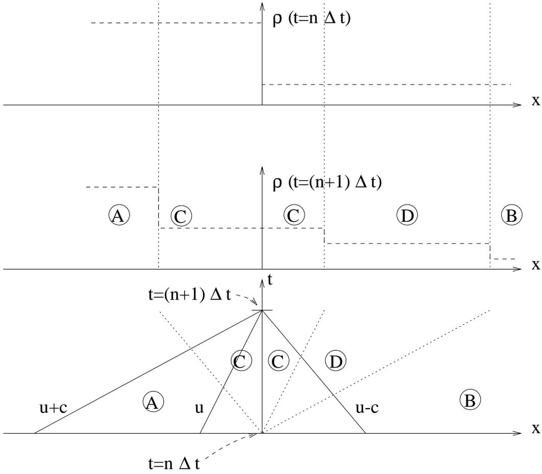
Figure 19: Characteristic based Riemann solver.
