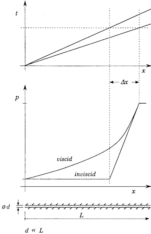
Figure 11: Sketch of an expansion wave in a long thin tube.
