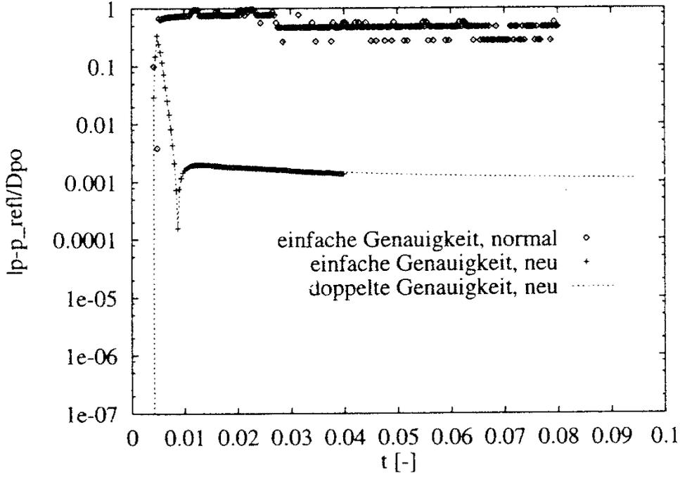
Figure 12: Error of computed pressure at an  $x$  location for  $M = 10^{-6}$ ,  $\diamond$ : conservative formulation and single precision,  $+$ : perturbation formulation and single precision,  $\cdots$ : perturbation formulation and double precision.
