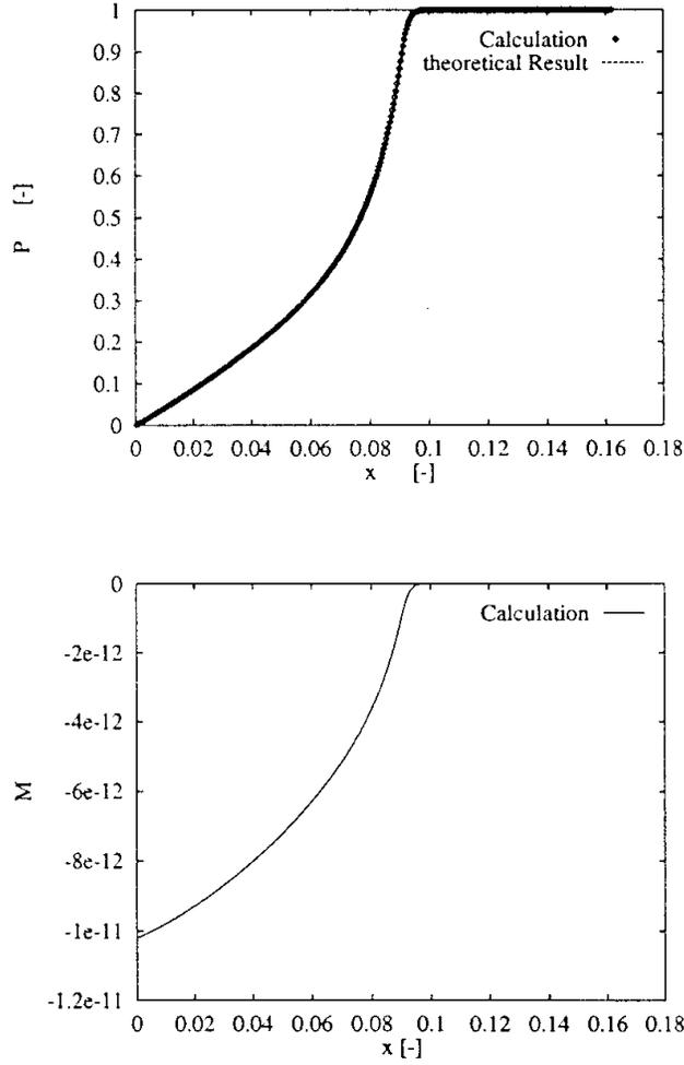
Figure 20: Pressure and Mach number at a time instant for  $M = 10^{-11}$ ,  $\diamond$  and solid line: computed result with perturbation formulation and single precision, dashed line: analytical solution.
