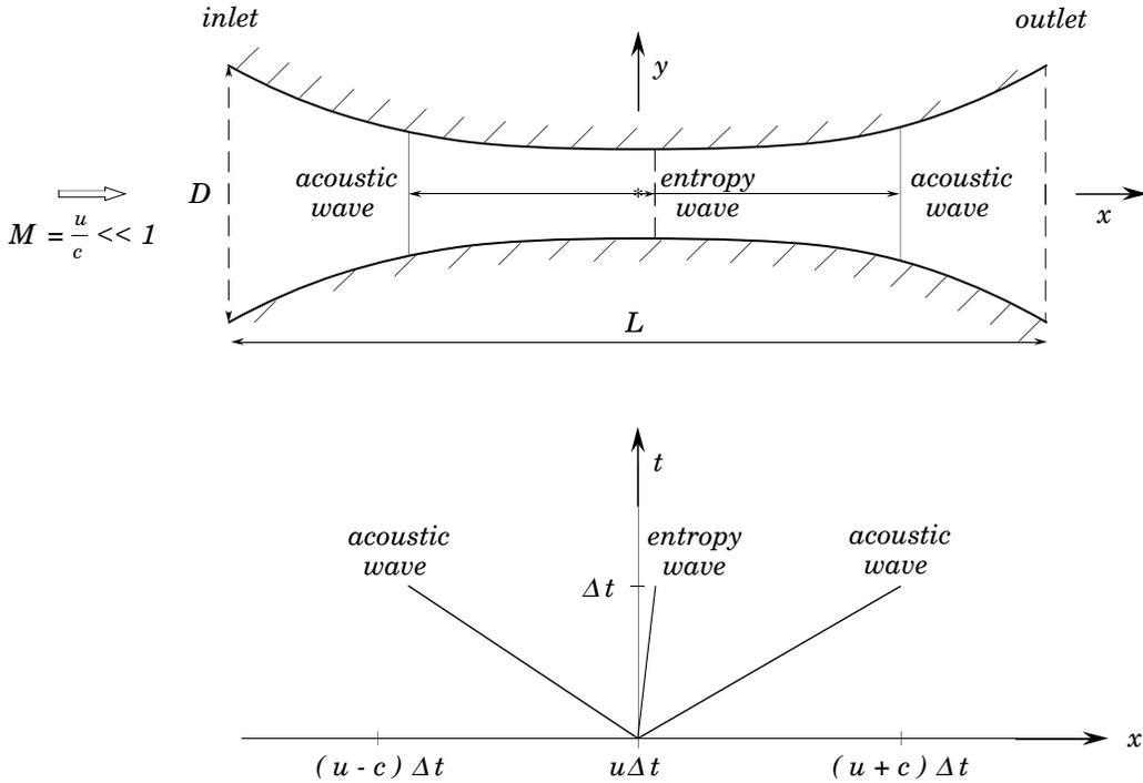
Figure 4: Acoustic and entropy waves generated by disturbance at  $x = 0$  after time  $\Delta t$  for low Mach number  $M$ .
