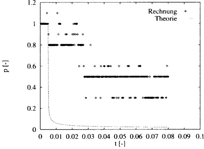
Figure 13: Pressure at an  $x$  location for  $M = 10^{-6}$ ,  $\diamond$ : computed result with conservative formulation and single precision,  $\cdots$ : analytical solution.
