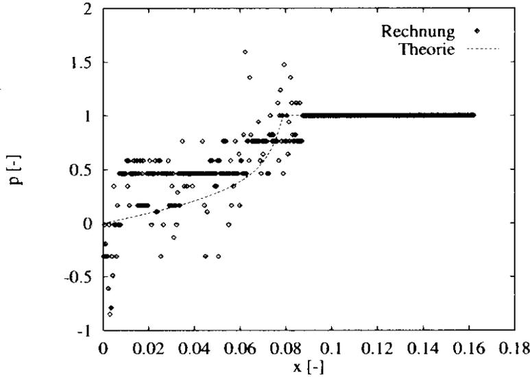
Figure 14: Pressure at a time instant for  $M = 10^{-6}$ ,  $\diamond$ : computed result with conservative formulation and single precision,  $\cdots$ : analytical solution.
