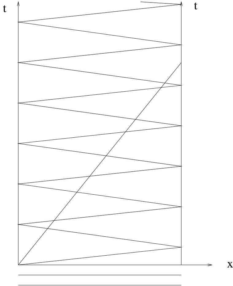
Figure 7: Reflection of acoustic waves at outlet and inlet in low Mach number flow.
