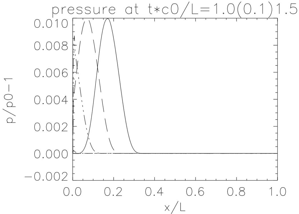
Figure 9: Acoustic pressure for acoustic pulse leaving the inlet computed with non-reflecting boundary conditions.
