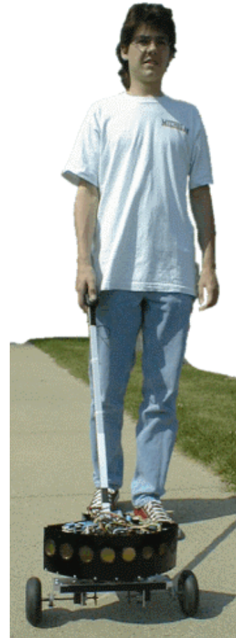
Figure 5: Iwan Ulrich demonstrates the actual GuideCane prototype.
