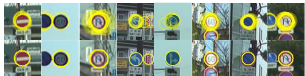
Figure 1: Output of the Hough circle detector before (upper row) and after (lower row) applying the Confidence-Weighted Mean Shift refinement procedure. The transparency of the detected circles in the upper row images correspond to their confidence expressed with the scaled number of votes picked from the Hough voting space.
