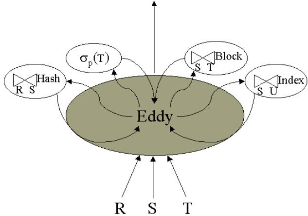
Figure 1: An eddy in a pipeline. Data flows into the eddy from input relations  $R$ ,  $S$  and  $T$ . The eddy routes tuples to pipelining operators; the operators run as independent threads, returning tuples to the eddy. The eddy sends a tuple to the output only when it has been handled by all the operators. The eddy adaptively chooses an order to route each tuple through the operators.
