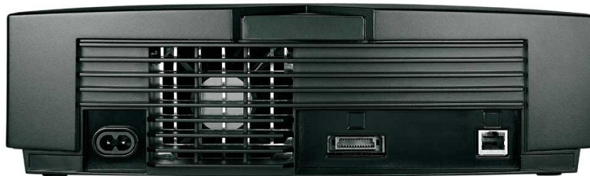
Figure 1.2: Xbox rear view: power supply connector, cooling fan, A/V connector, ethernet port
