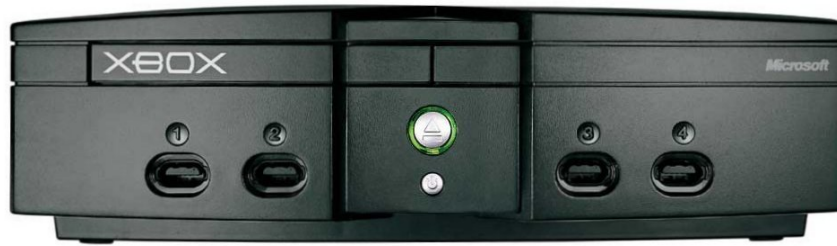
Figure 1.1: Xbox front view: DVD tray (with Xbox font on it), four USB 1.1 ports, power button (below) and the eject DVD button (with the LED surrounding it)
