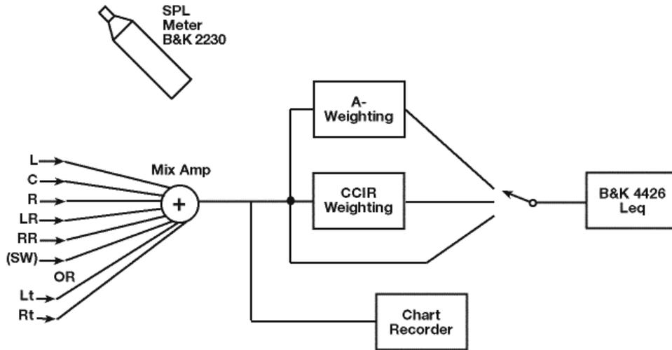
**Figure 3** Test set-up
