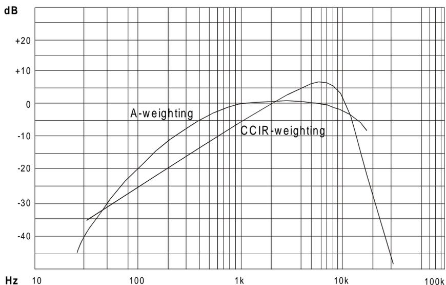
**Figure 4** A-weighting vs. CCIR-weighting curve (offset by 5.6 dB)
