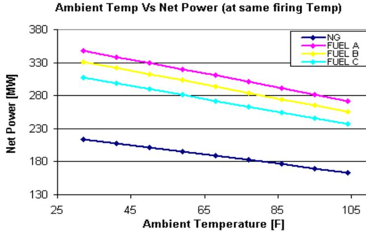
Figure 4. Influence of ambient temperature on power output at the same firing temperature
