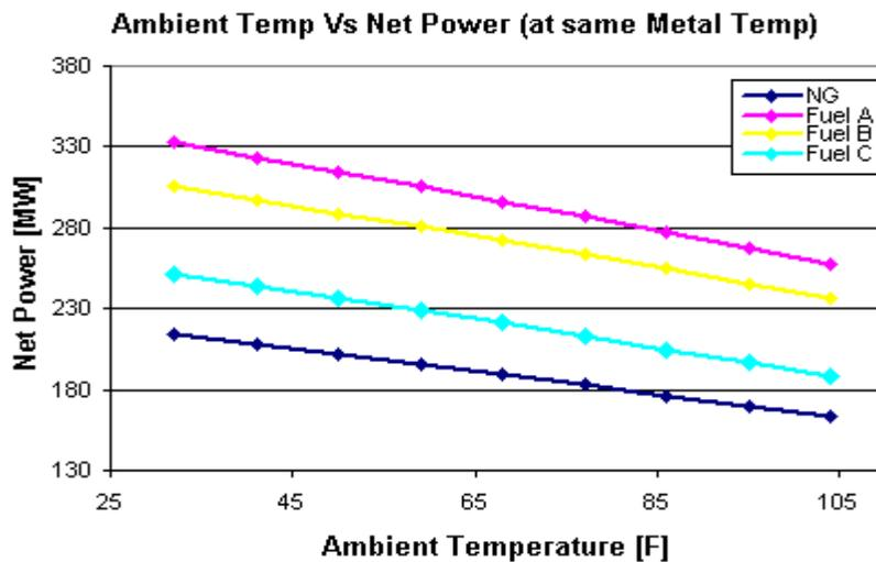
Figure 3. Influence of ambient temperature on power output at same metal temperature
