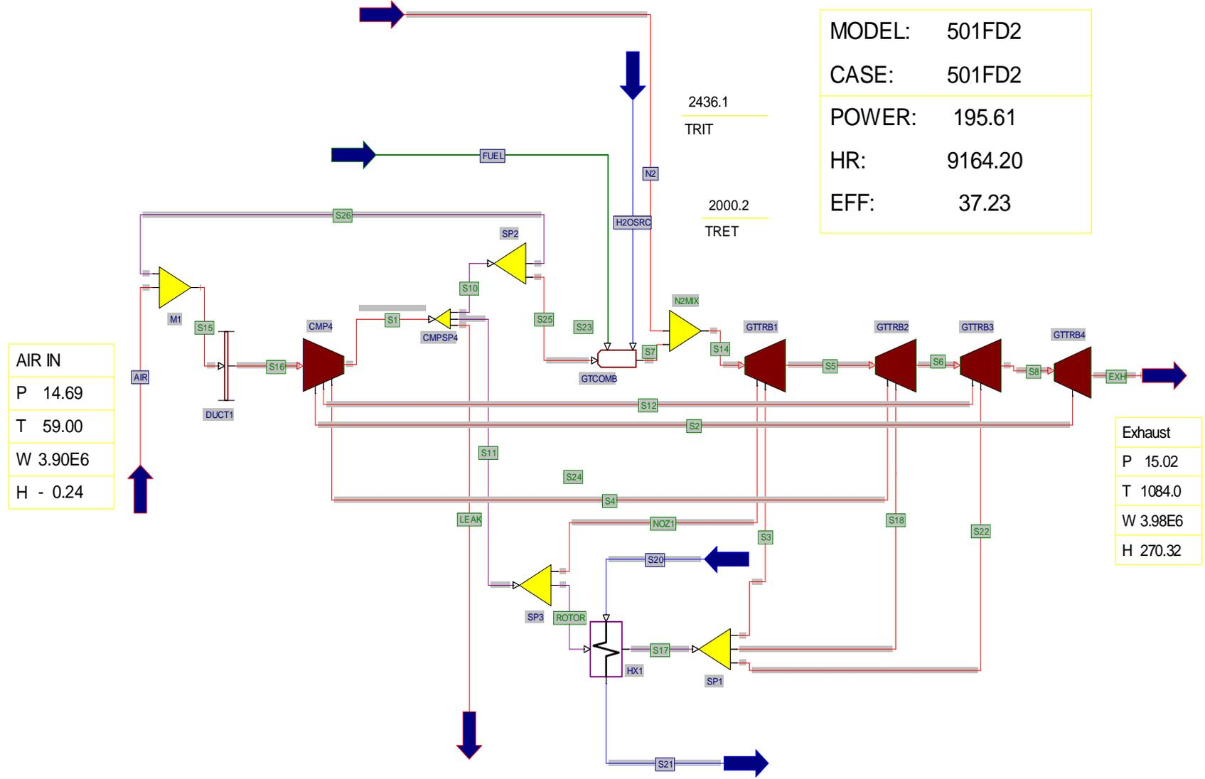
Figure 2. Block diagram showing design conditions for natural gas
