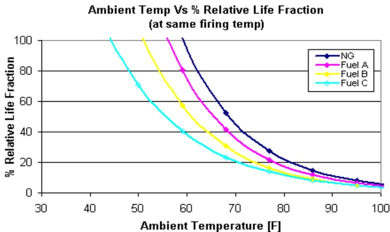
Figure 5. Relative life of turbine hot sections fired with different fuels.
