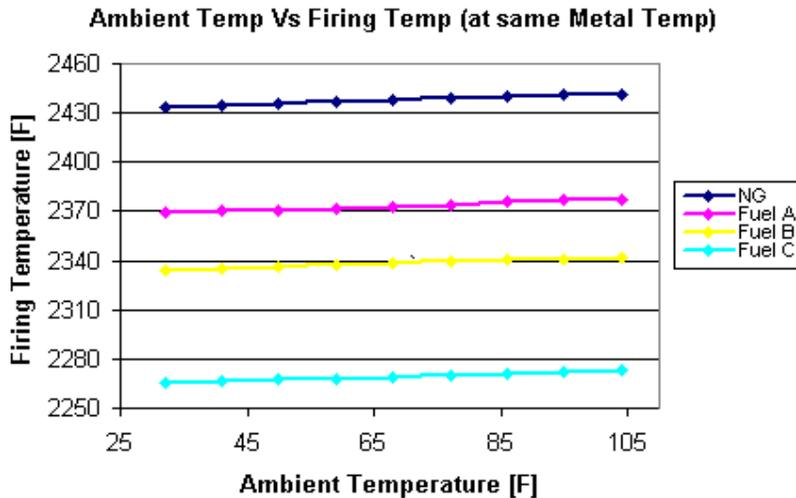
Figure 6. Derated firing temperature necessary to maintain metal temperature
