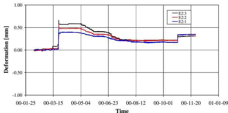
Fig. 12. Recorded deformation along extensometer E2. Positive deformation corresponds to extension. The units are in mm.
