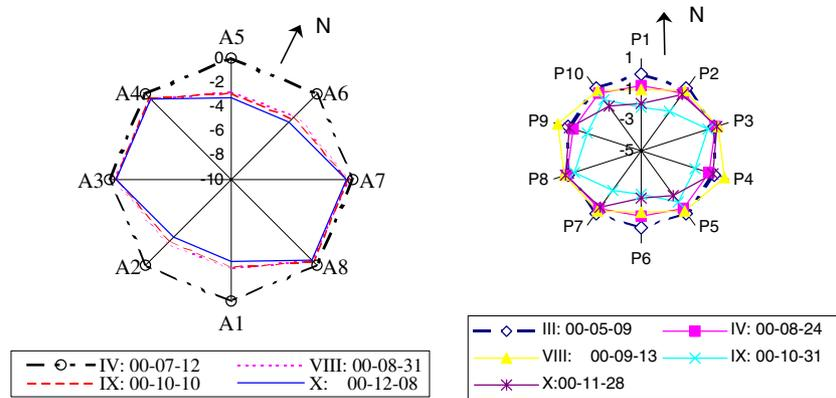
Fig. 11. Recorded cavern convergence during the excavation. To the left is shown convergence in the upper niche and to the right convergence in the cavern roof. The units are in mm.
