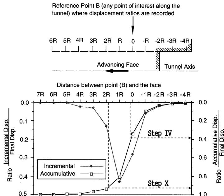
Fig. A1. Radial displacement of a reference point (B) associated with tunnel face advance for an unlined tunnel under elastic conditions (modified after Hanafy, 1980).
