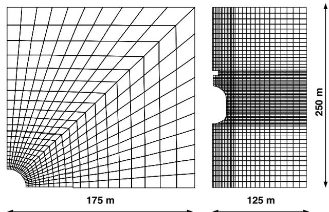
Fig. 9. The element grids used in the numerical calculation. To the left is shown the horizontal plane at the cavern upper niche (LRC10) and to the right the axi-symmetric vertical section of the cavern (LRC20 & 30).
