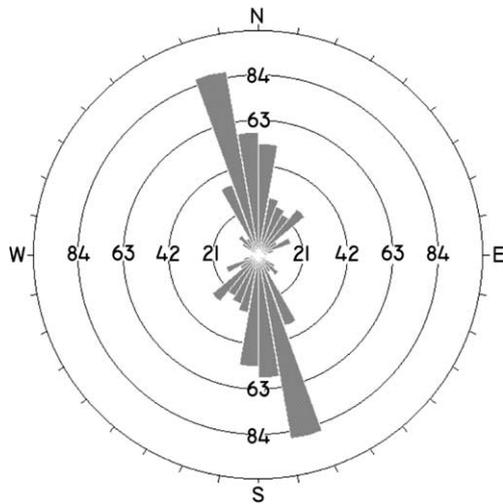
Fig. 5. Joint rose diagram showing the strike of the dominating joint sets based of approximately 400 joint planes mapped in the cavern.
