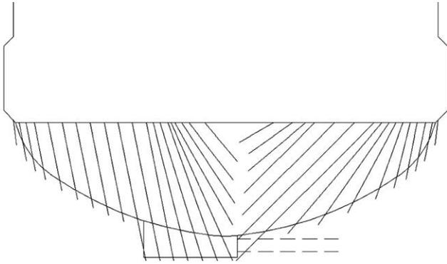
Fig. 8. Vertical section of the cavern bottom showing the drill pattern of the bottom excavation (after Allvin et al., 2001).
