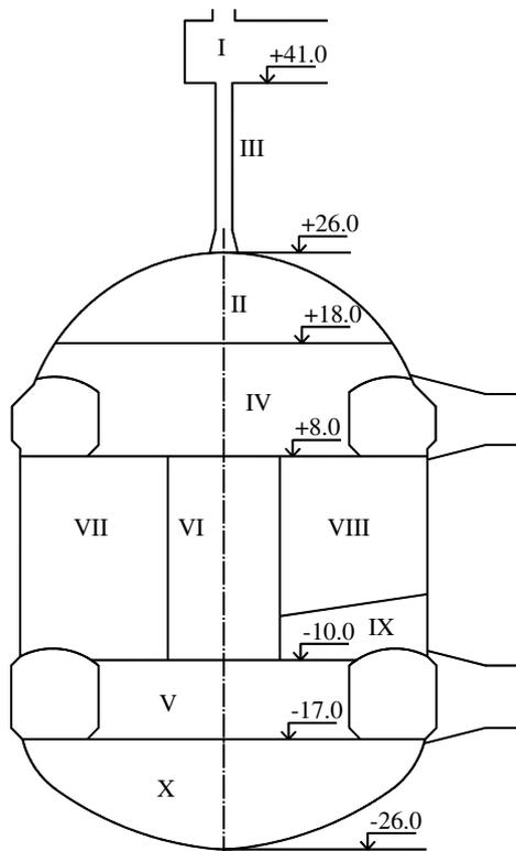
Fig. 6. Vertical section of the cavern showing the steps and levels in the excavation sequence. Ground surface on level +135.
