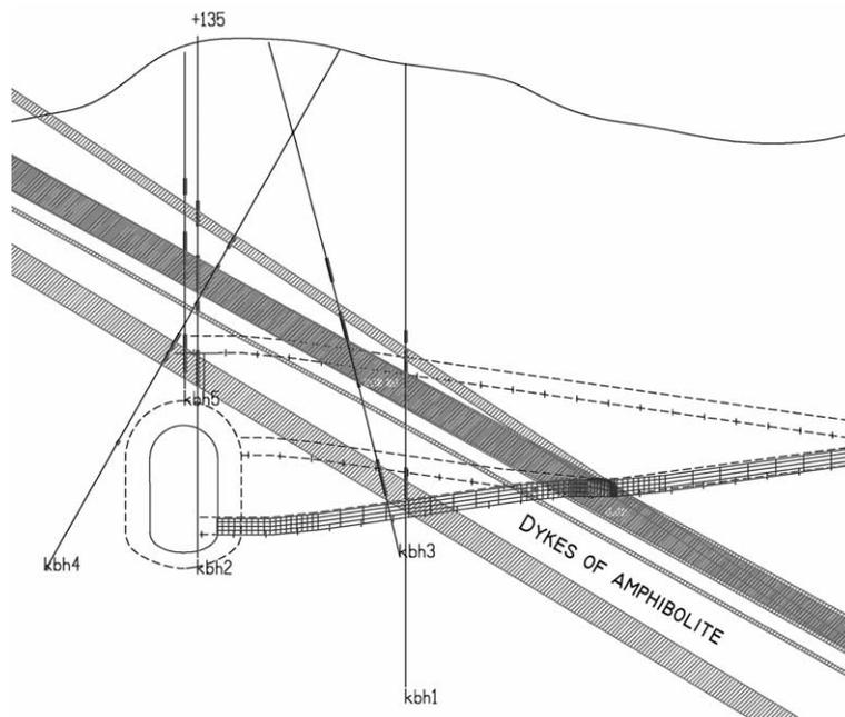
Fig. 3. Geological model of the site in west-east direction there the amphibolite dikes are shaded. The model is interpreted from five core drillholes and mapping along the access tunnels.
