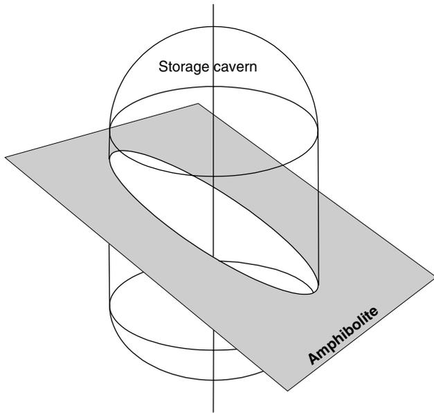
Fig. 4. Location of the Amphibolite dike encountered within the cavern.
