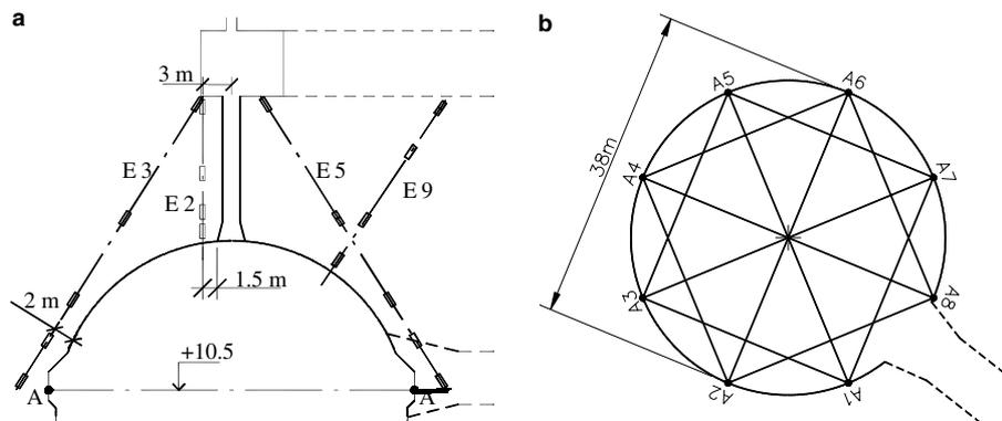
Fig. 10. Positioning of convergence measurements in the cavern (series A) and extensometers around the cupola (series E).
