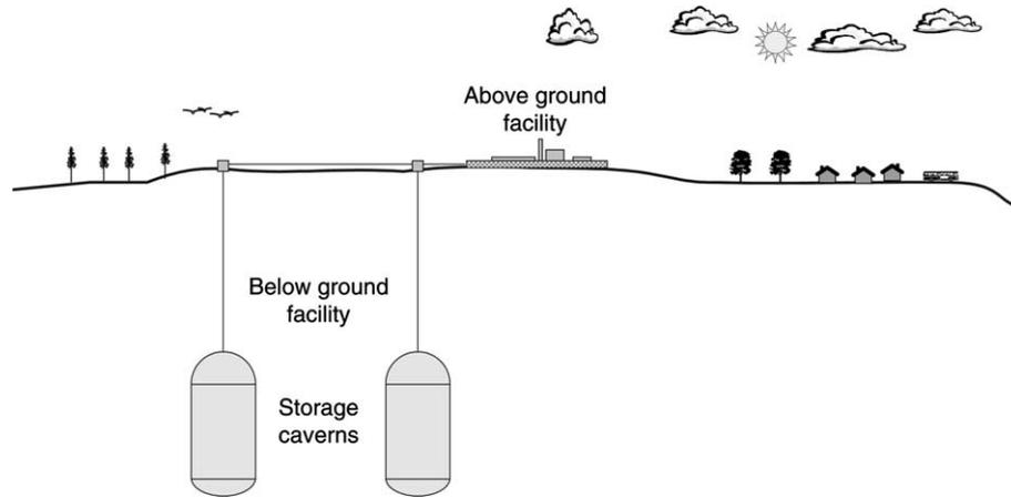
Fig. 1. Schematic illustration of an LRC gas storage plant (after Johansson, 2003).
