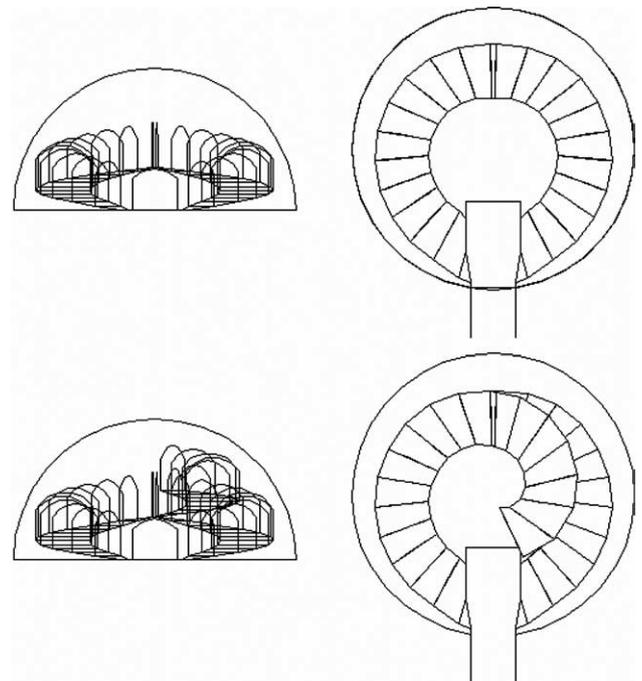
Fig. 7. Schematic illustration of the cavern crown excavation. Upper part showing the spiral tunnels and the bottom part the ramp in the cupola (after Allvin et al., 2001).
