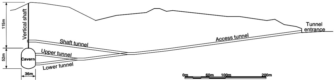
Fig. 2. Layout of storage cavern and access tunnels at the LRC Demo Plant (after Johansson, 2003).
