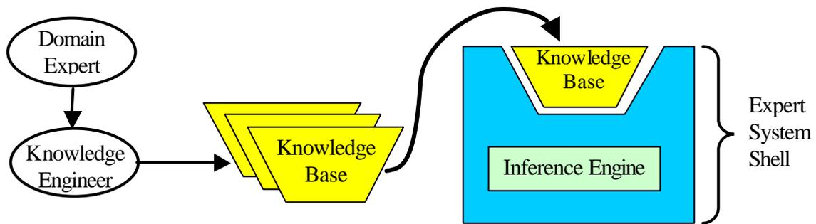
**Figure 2.** Expert system development from a reusable shell and knowledge bases.
