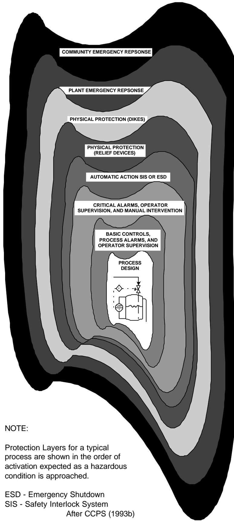
**Figure 1: Typical Layers of Protection for a Chemical Manufacturing Process**
