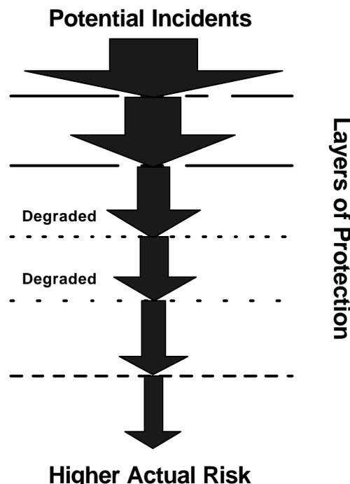
**Figure 3: Reduced Effectiveness of Degraded Layers of Protection**
