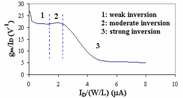
Fig. 3  $g_m/I_D$  as a function of  $I_D/(W/L)$
