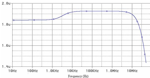
Fig. 5 OTA's transconductance in weak inversion region
