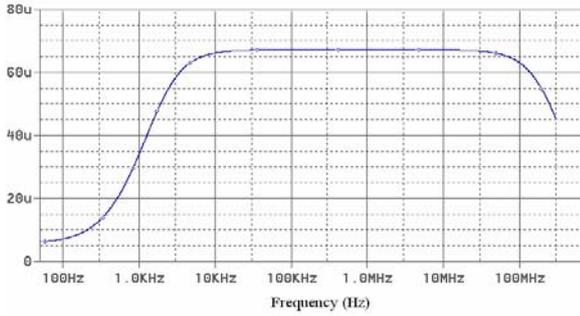
Fig. 7 OTA's transconductance in moderate inversion region
