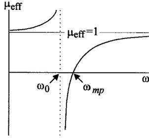
Fig. 5. The effective magnetic permeability for model *B* shows a resonant structure dictated by the capacitance between the sheets and magnetic inductance of the cylinder. We sketch the typical form of a highly conducting sample,  $\sigma \approx 0$ . Below the resonant frequency,  $\mu_{\text{eff}}$  is enhanced, but above resonance,  $\mu_{\text{eff}}$  is less than unity and may be negatively close to the resonance.
