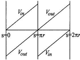
Fig. 16. The emf acting around one of the sheets of the split ring in Fig. 12 as a function of the distance  $s$  around the ring.  $V_{in}$  denotes the emf on the inner ring, and  $V_{out}$  that on the outer ring. Note that this ring is cut at  $s = 0$  so that the emf is discontinuous.
