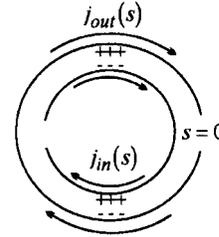
Fig. 4. When a magnetic field parallel to the cylinder is switched on it induces currents in the “split rings,” as shown here. The greater the capacitance between the sheets, the greater the current.
