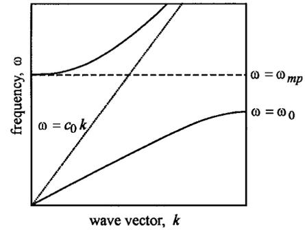
Fig. 6. Generic dispersion relationship for resonant structures with a  $\mu_{\text{eff}}$ . The solid lines represent twofold degenerate transverse modes and the dashed line a single longitudinal magnetic plasmon mode.
