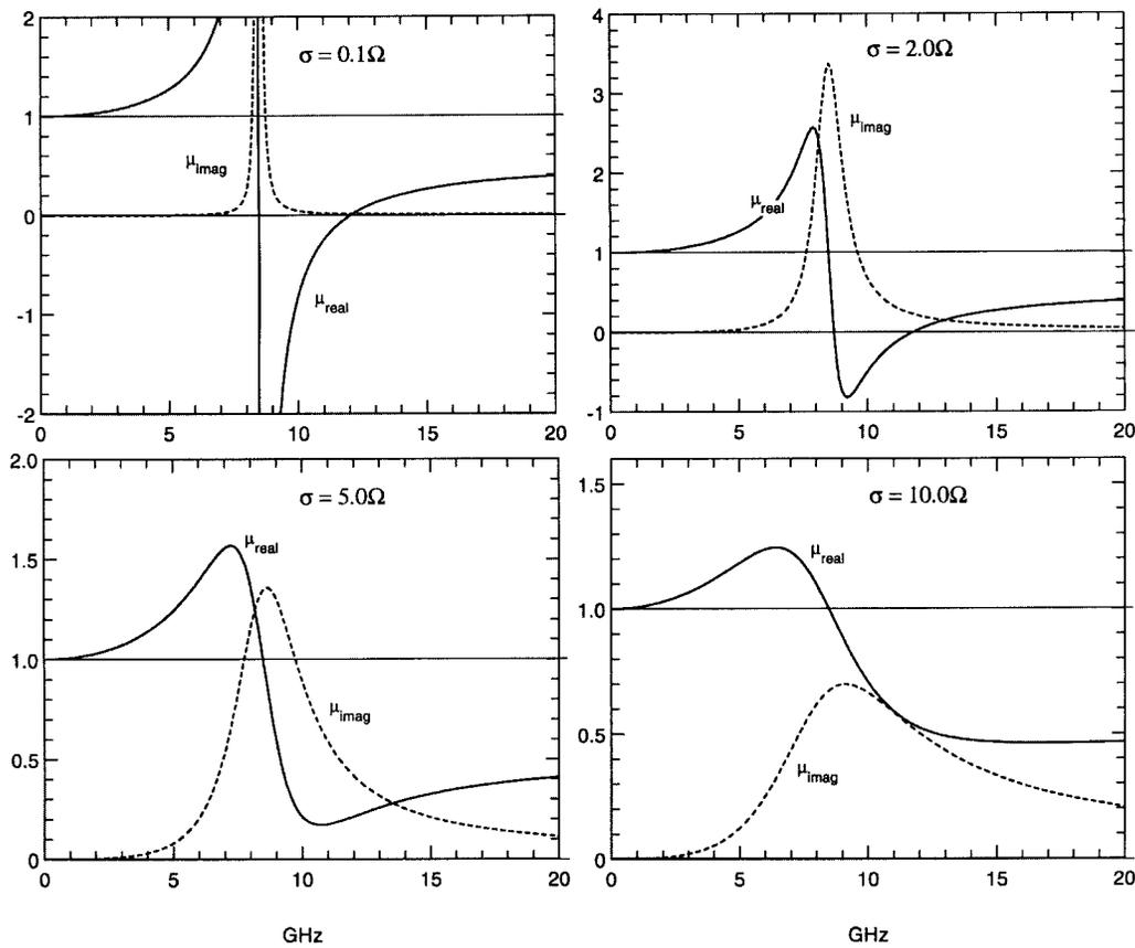
Fig. 10. Dispersion with frequency of  $\mu_{\text{eff}}$  for a Swiss roll structure, calculated for the parameters shown in (36), for various values of the resistivity of the sheets: 0.1, 2.0, 5.0, 10.0  $\Omega$ .
