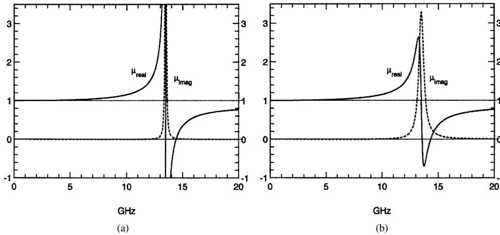
Fig. 15. Plot of  $\mu_{\text{eff}}$  for the cubic split ring structure calculated using the chosen parameters. (a) For copper rings,  $\sigma_1 = 200.0$ . (b) For more resistive rings,  $\sigma_1 = 2000.0$ .
