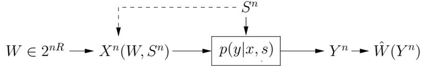
Figure 2: Channel with non-causal transmitter side information
