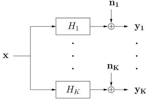
Figure 1: The vector broadcast channel
