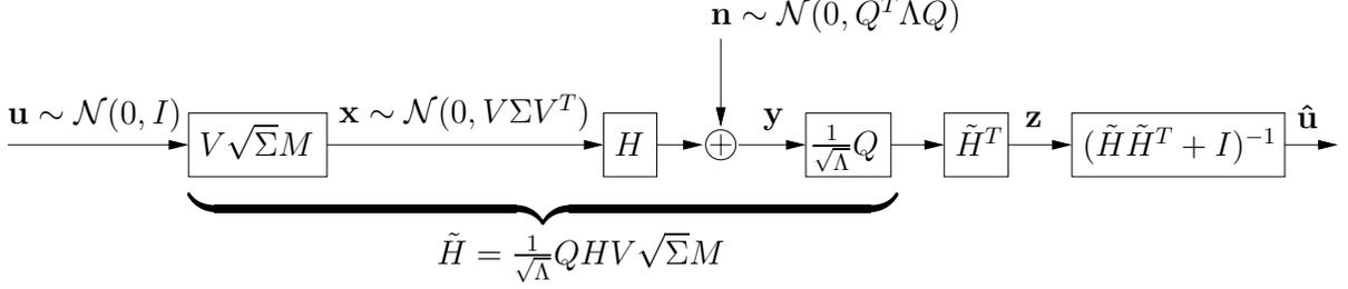
Figure 11: GDFE with transmit filter
