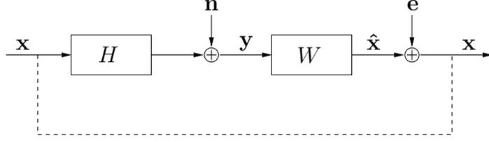
Figure 5: Minimum mean-square error estimation
