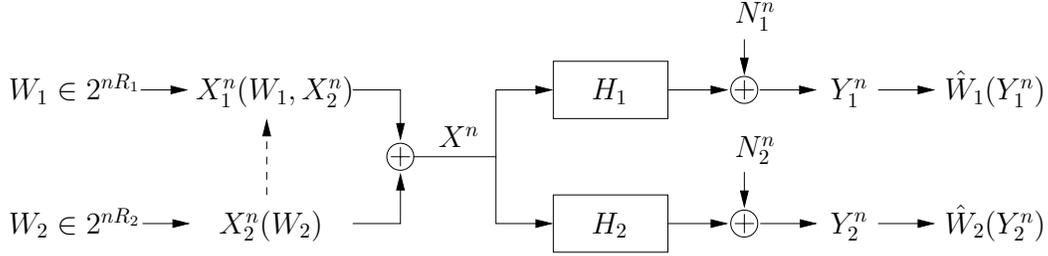
Figure 4: Coding for vector broadcast channel
