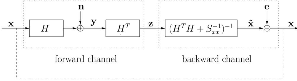
Figure 6: Forward and backward channels
