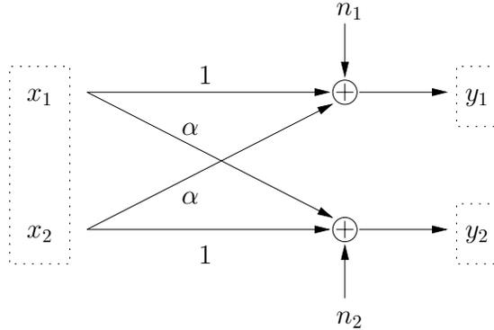
Figure 10: A two-user broadcast channel
